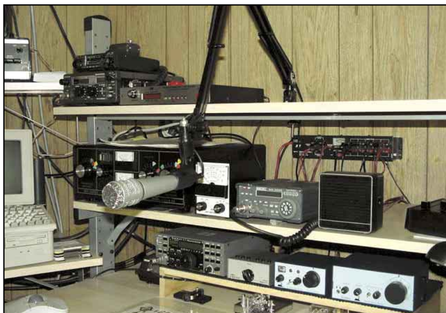
Figure 1—Installed on an articulated lamp arm, the modified RadioShack mike provides me with a professional looking (and great-sounding) means of making QRP phone contacts.
