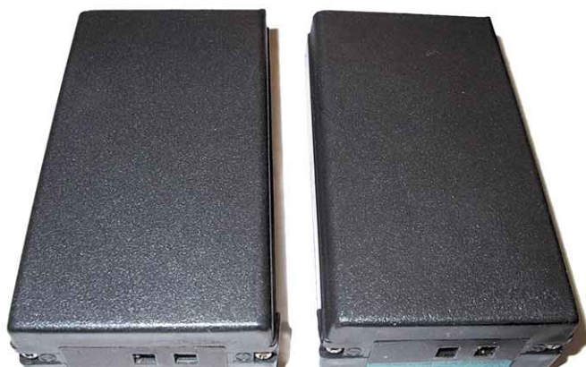
Figure 2—Two 13.8-V battery packs for my ICOM IC-2GAT H-T. The pack on the left is an older NiCd unit having a rating of 1200 mAh. The one on the right is an NiMH with a rating of 2700 mAh. They have identical case sizes.
