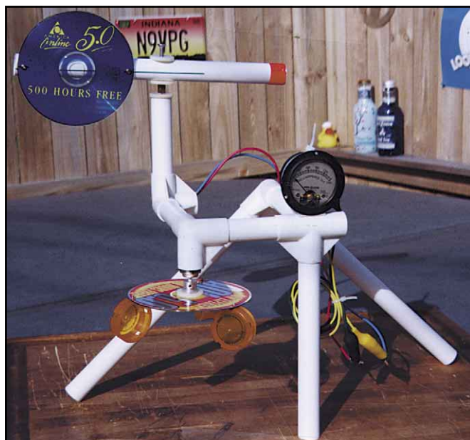
Figure 1—N9PUG's junk-box anemometer for stingy meteorologists. The horizontal CD (at left below center) is the anemometer. The horizontal pipe and CD at the top form a weather vane for visual observation. (Perhaps readers could adapt rotator direction sensors for remote reading or develop new techniques for the task. Send in the hints!—Ed.) The wind-speed meter is cleverly mounted to the pipe at center, but it would normally be located conveniently indoors. Although Greg made this complex PVC arrangement to stand on its own, one made for roof or tower installation could be much simpler, as fewer legs and bends are needed.
