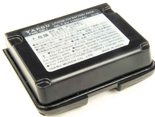
Figure 5—Small Li-ion battery pack for the Yaesu VX-5R H-T.
