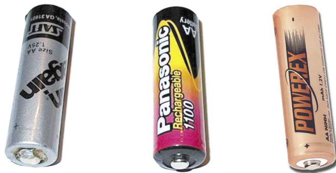
Figure 3—Three different types of AA-size cells. At left, an older NiCd cell rated at about 600 mAh; in the middle, a newer NiCd cell with an 1100 mAh rating; at the right, an NiMH cell rated at 1600 mAh. Note that 1300 mAh is a "comfortable" rating for an NiMH cell of this size; higher capacity cells are readily available.
