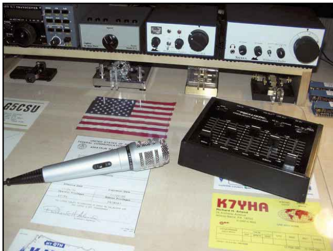
Figure 2—My RadioShack mike ($19.95) and Amp/EQ unit—a simple and inexpensive means of enhancing transmitted audio on QRP phone.
