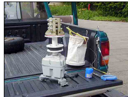
The big arrays were lurching rotators until the W6UE gang came up with this custom flex drive setup. Problem solved!
