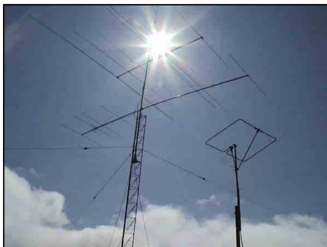
The 6-meter antenna presently set up at HC8N is an M 2 6M7JHV Yagi. The 6-meter halo in the foreground serves as the antenna for the HC8GR beacon.
