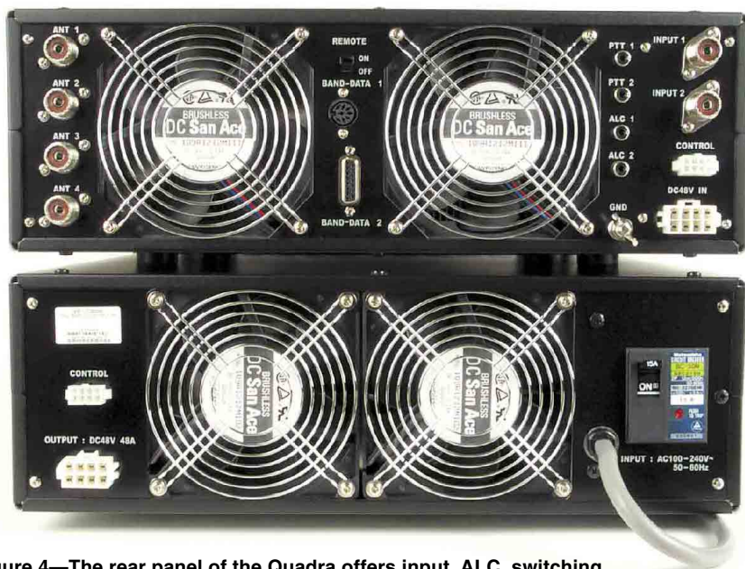
Figure 4—The rear panel of the Quadra offers input, ALC, switching and control connectors for two separate exciters and outputs for up to four antennas.
