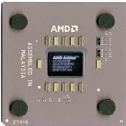
The business end of a 1.3-GHz AMD CPU. The four rubber pads prevent the heat sink from tipping to one side or another, which would compromise the heat transfer from the already small contact patch (center).
