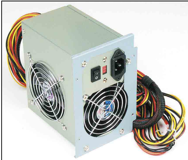
High-power PCs require beefy power supplies. This 450-W Enermax unit has thermostatically controlled fans and extra-long cables to accommodate large cases. Need more? Go with its 650-W big brother!
