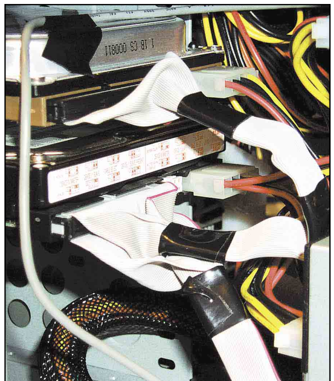
What to do with pesky IDE cables? The new high-performance cables designed for UDMA 66 and UDMA 100 drives fold up rather nicely. The compact cables provide for a tidy layout and less-restricted air flow.
