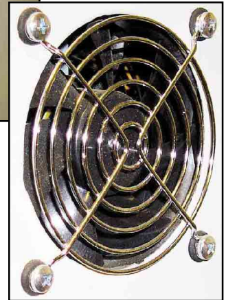
A close-up of the "blowhole." The rubber grommets greatly reduce noise and vibration.
