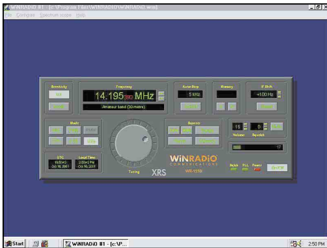
Figure 1—The virtual front panel of the WinRADiO WR-1500i communications receiver. Don't let its simple appearance fool you—this receiver is packed with sophisticated capabilities.
