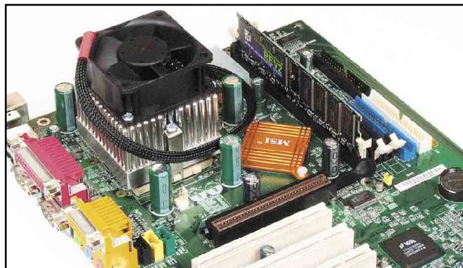
The innards of the Project PC. The motherboard is an MSI K7T Turbo (with a KT133A chipset). Note the ATX-style I/O connectors at the lower left. At the right is a 256-MB stick of Mushkin REV2 high-performance SDRAM and, nestled underneath the massive Swiftech MC-370 CPU cooler lurks a 1.3-GHz AMD Thunderbird processor. This has proven to be a nice combination. (All photos in this article by the author.)
