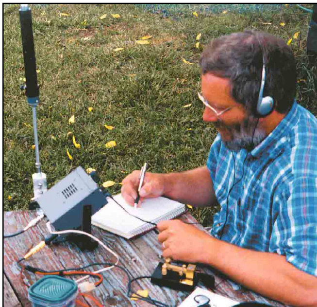
The author operates his 7-W CW station: Elecraft K1 QRP transceiver, Super Antennas MP-1 HF portable antenna and Kent single-paddle key.
