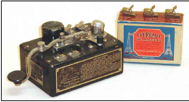
This 1918 practice set was made for training operators during WW-I. It had a light and a buzzer and could be connected to others via external wiring and using a battery like that shown. Hams bought these from surplus companies after the war. Note the extension on the key to bring the knob down to regular height.
