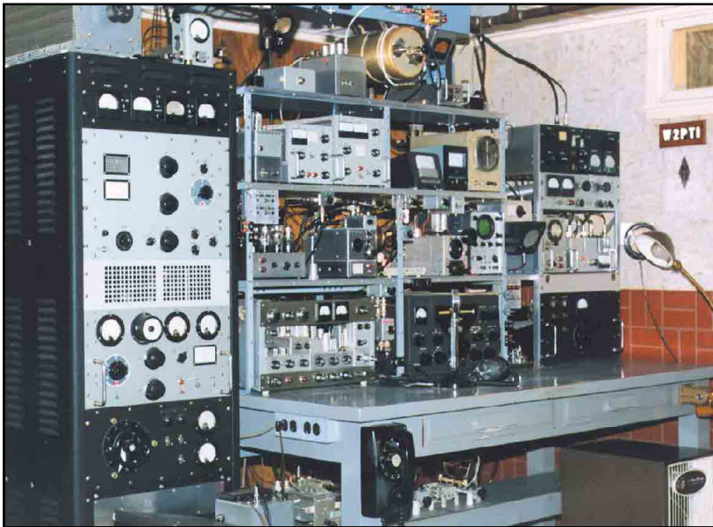
"Thought you might want to see some homebrew," writes Francis A. Waggoner, W2PTI, of Watertown, New York. For those who haven't been able to figure it out from the photo, you're looking at: 4-1000 amp, 4CX1000 amp, 0-4000 V dc power supply, SSB exciter for 10-15-20-40-80, 160-m transverter, 160-m amp (two 4X250s), 2-m converter by W2AZL, 2-m transverter, 2-m amp (also two 4X250s), 70-cm transverter, 70-cm amp (4X250), 0-2000 V dc power supply, and a 75-A4 receiver. The latter, Francis admits, isn't homebrew. In fact, you can see the first of these famous Collins receivers (serial no. 000001) at ARRL Headquarters.
