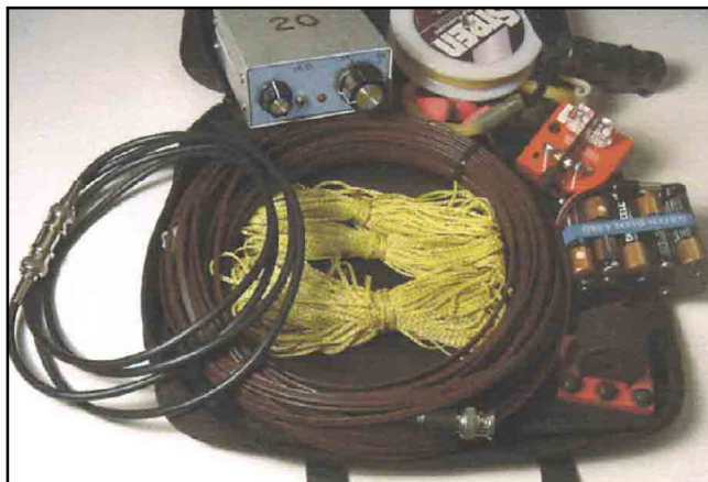
Figure 2—The author's portable station, including twin-lead dipole, 20-meter Wilderness Radio SST transceiver and support line. It all fits in the 8"x10 1/2"x2" Compaq notebook computer case.
