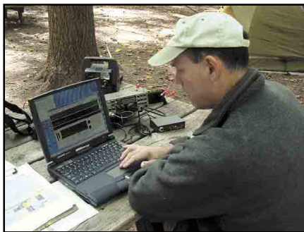
Figure 3—Ed Breneiser, WA3WSJ, is using his laptop running WinPSKse software and his Elecraft K2 transceiver to enjoy some PSK31 operating from a camp site in French Creek State Park, near Reading, Pennsylvania. The ability to use this station from almost any location has a direct application in emergency communications applications.
