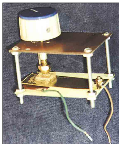
Figure 3—A photo of the prototype 2-pF (1x3-inch brass strip) compression capacitor.
