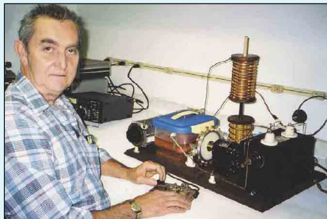
David Wilson, VE3BBN, demonstrates his rotary spark gap transmitter.
