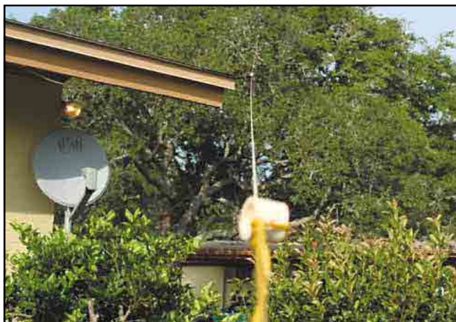
An end-on view of the N2CX Gusher 40 meter portable dipole, looking “up” the antenna from the swing set in the backyard into the tree. This antenna withstood 70+ mph winds during Almost-Hurricane Barry at Tyndall AFB, Florida.
