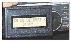
and watch the decoded copy scroll across the LCD. The device locks on and tracks code elements up to 99 words per minute.
