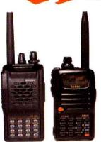
FT-50RD/41B Commercial-grade, military spec. It's rugged, reasonably priced, and simple to operate. Boasting 5 Watts output power, the 50RD covers 144 and 430MHz while also offering the "widest" band receive allowable.
