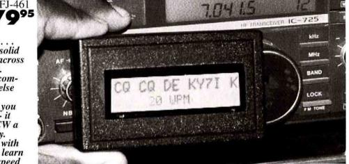
4. Both top and bottom lines scroll. Two-line LCD display has 32 large 1/4 inch high-contrast characters.
