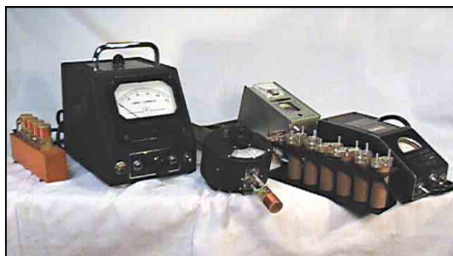
Figure 1—Several common types of dip meters are shown with their plug-in coils that determine the oscillator’s frequency.
