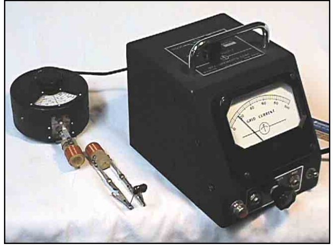
Figure 5—Tune the dip meter's frequency until the unit's meter reaches a minimum—or "dips." The plug-in coil is attached to the capacitor with slide-on alligator clips.
