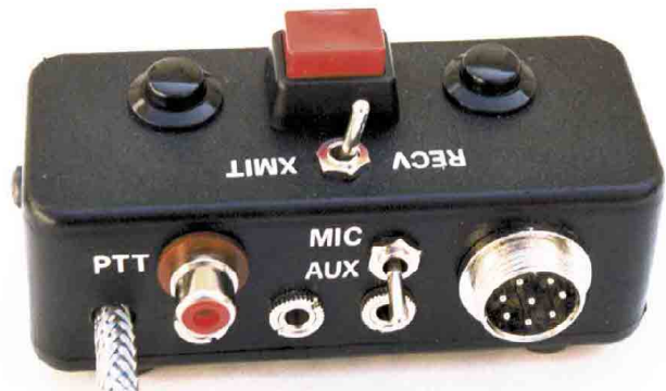
Figure 5—The rear/top view of the adapter shows the button, switches and connectors.
