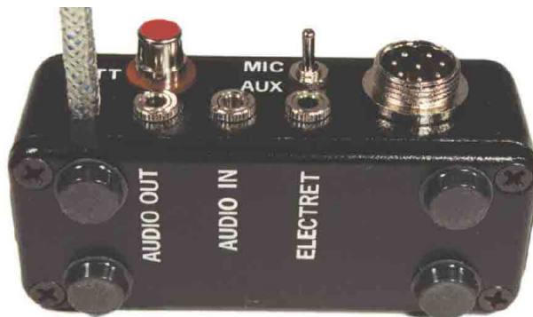
Figure 5—The rear/top view of the adapter shows the button, switches and connectors.
