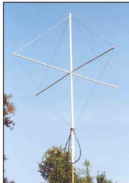
An overall view of the quad-turnstile on the assembly and test stand. I took this photo during initial tests before adding the perimeter cord and taping down the phasing line and feed line.
