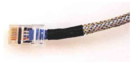
Figure 3—The adapter's mike cable (a piece of RJ-45 LAN cable) is shielded with braid from a piece of RG-58 coax and fixed in position with heat-shrink tubing.
