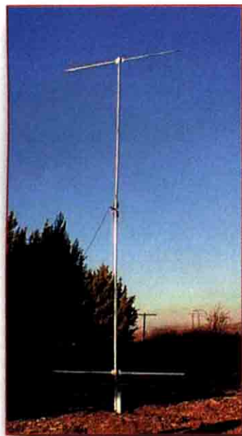
Sigma-40™ 40 meter vertical (24' tall, free standing, 38 lbs.)
