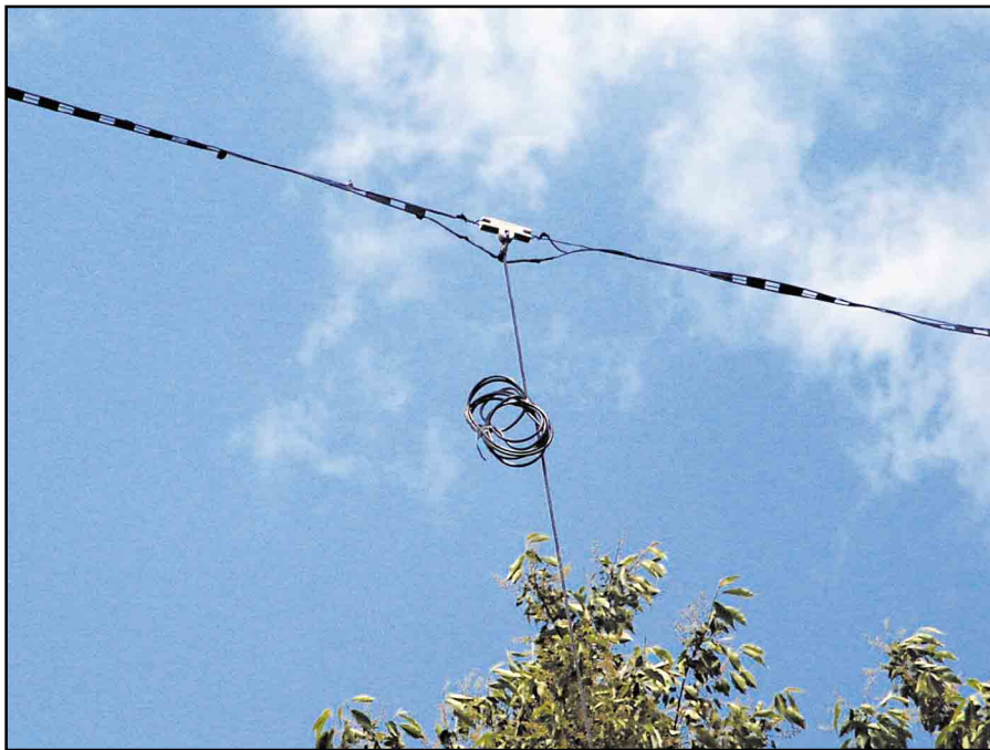
Figure 7— The K4VX 40-meter linear-loaded dipole deployed at 40 feet.
