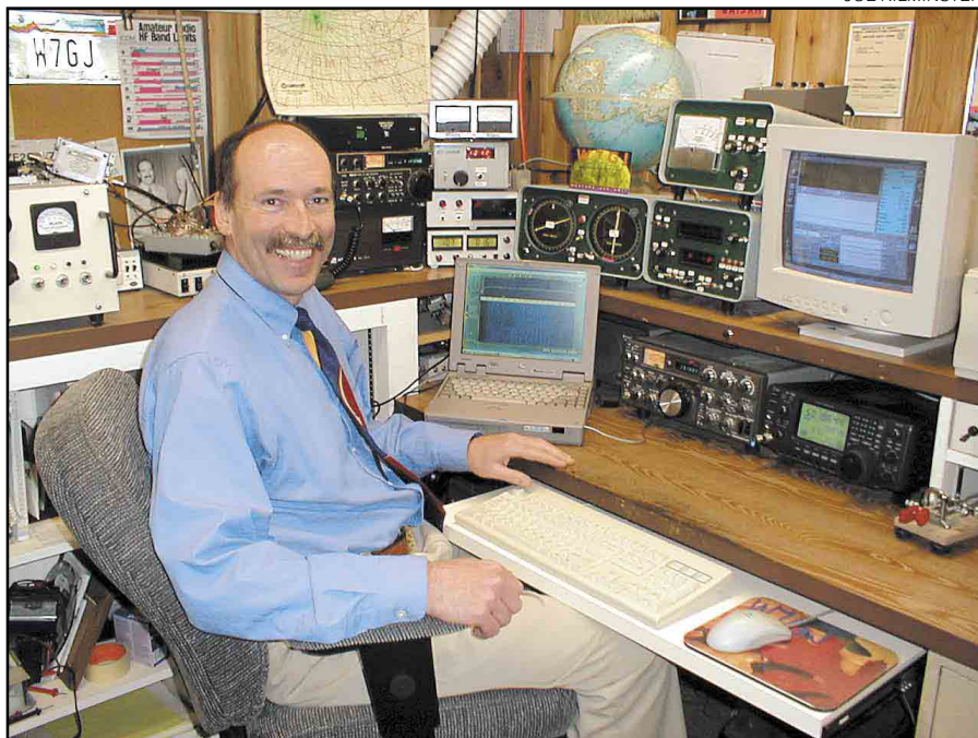
Lance Collister, W7GJ, in his neatly arranged shack at Frenchtown, Montana. Lance monitors weak signals visually using Spectran on a laptop computer, while JT44 runs on the second computer.
