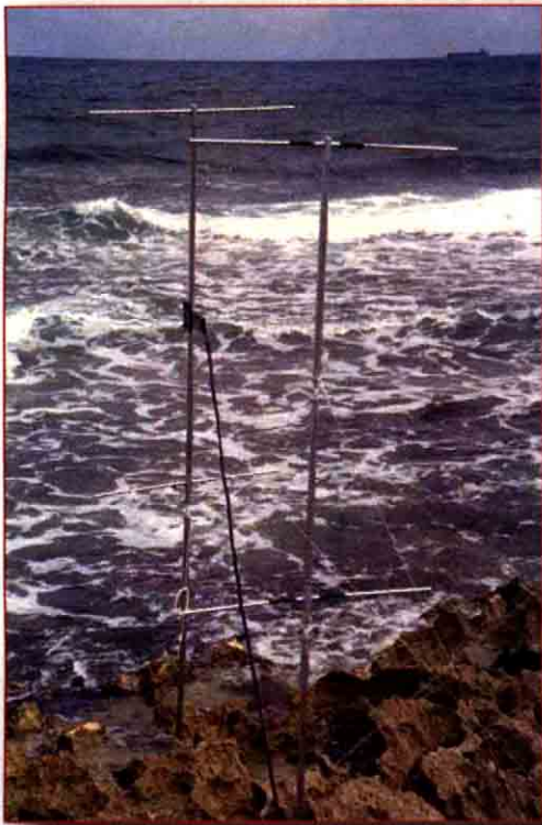
Sigma-6™ 6 meter band full vertical (6' tall + base, 6 lbs.)
