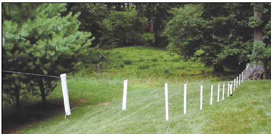
Figure 5—A tri-band N4GG Array stretched out 3 feet above the ground for easy assembly. Half-inch PVC spreaders are used to separate the wires by 4 inches.
