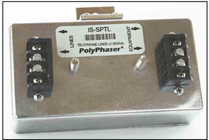
Figure 9—A telephone line protector.
