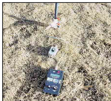
Figure 12—Finding the permanent adjustment points on the coil for each band.
