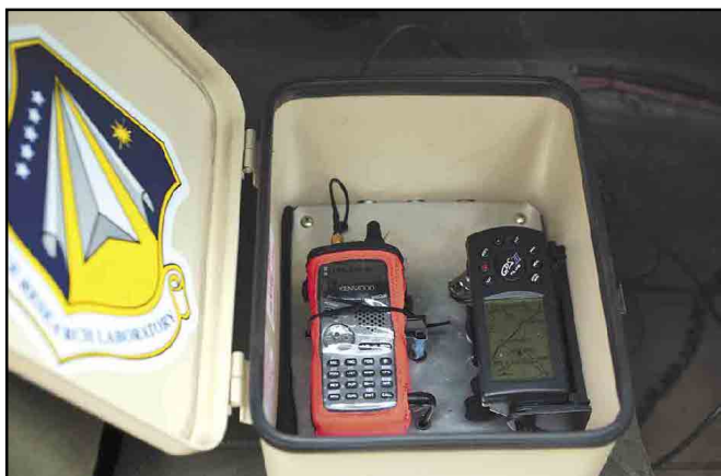
Figure 1—The PEAPRS station consisted of a Kenwood TH-D7 handheld transceiver and a Garmin GPS III Plus GPS receiver contained in a metal box. The GPS calculated the position of the aircraft and fed that data to the APRS software that is integral to the TH-D7.
