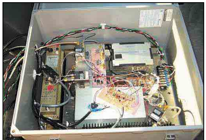
N1MU crafted this homebrew 10-GHz transverter.
