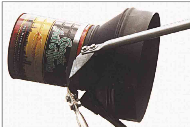
Since we intend to use the VSA at L-band, on a frequency of 1296 MHz, one can scale the dimensions of the standard C-band feed by a factor of three. As is the amateur tradition this feedhorn is constructed from low-cost materials!
