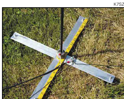
Close-up of the feedpoint of the HFp. When configured for 40 meters, the antenna stands 10 feet 6 inches high.
