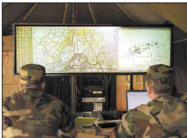
Figure 2—The map display of WinAPRS software was integrated into the large display inside the PEAPRS command tent.
