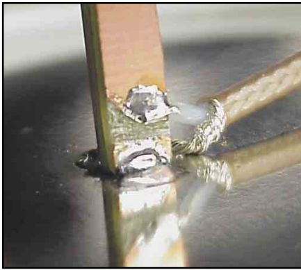
Figure 1—Close-up view of the coax connection to PCB transmission line and support.
