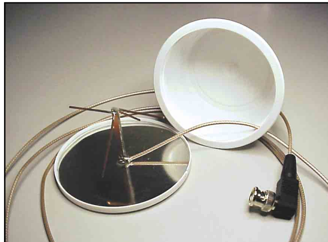
Figure 6—The finished GPS antenna with radome ready to snap into place.
