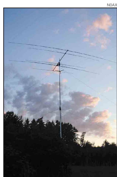
The WRTC teams all used these small tri-banders made by Oy Finnish Antennas Ltd, mounted on a 12-meter crank-up tower.
