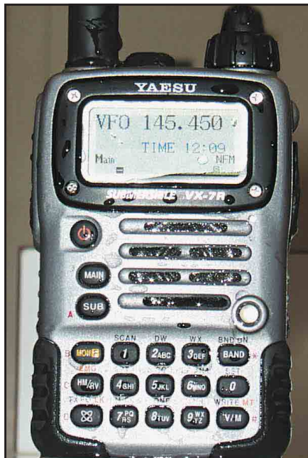
Figure 2 —Thirty minutes after being placed in 8.5 quarts of water, the Yaesu VX-7R, water dripping off its chassis, works like new.
