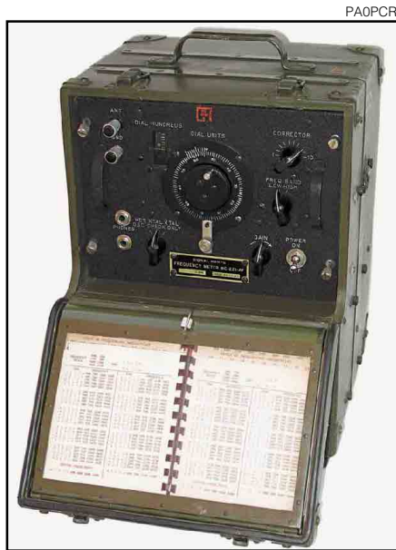
Figure 4—The SCR-221/BC-221 frequency meter, a precision instrument used in both military and civilian applications.
