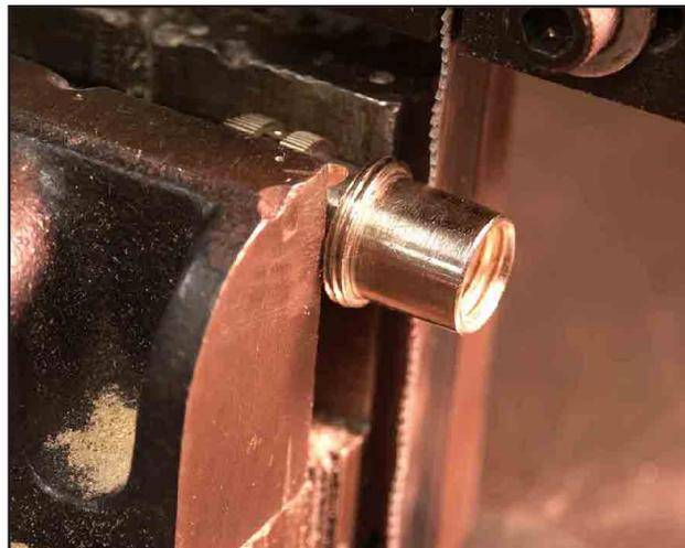
Fig B—Trim excess material from the rear of the PL-259.
