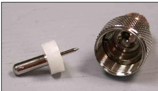
Fig 2—(above)The center-pin assembly is removed from the connector by securing the connector body in a vice, grasping the thick pin with pliers and pulling the assembly free.
