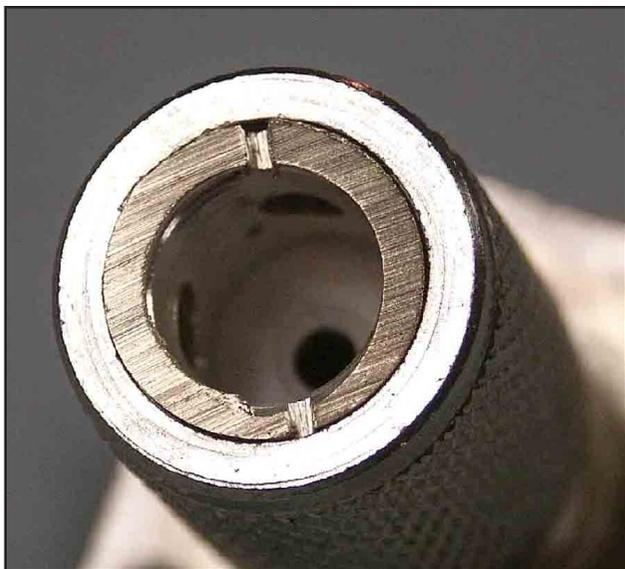
Fig C—(above) Here is the trimmed, sanded and notched PL-259. I trimmed too much; it would be better if the notched shoulder stood at least  $\frac{1}{16}$ -inch proud of the coupling ring. Fig D—(right) A finished SurCapAdapt PL-259 style. I used a stainless-steel screw that was on hand. With a brass screw, the wire could be soldered to the screw head, eliminating the second nut and solder lug.
