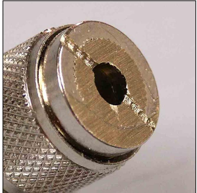
Fig 5—A shallow notch in the rear face of the connector serves to contact and hold the device under test.
