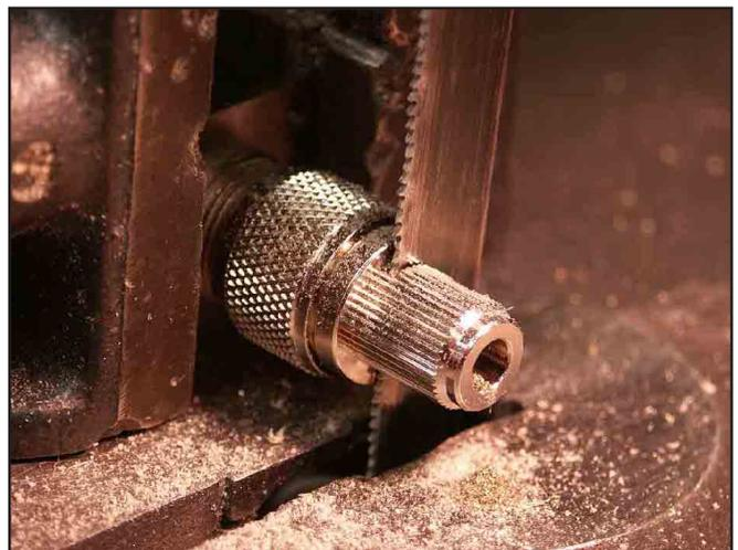
brass machine screw using a #55 drill bit. This hole must be drilled through the entire length of the screw body.
