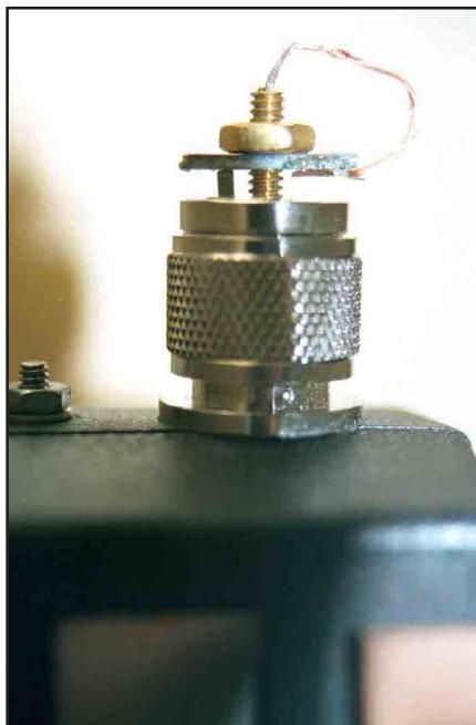
Fig 1—The author's SurCapAdapt mounted on the Autek RF-1 Analyzer.
