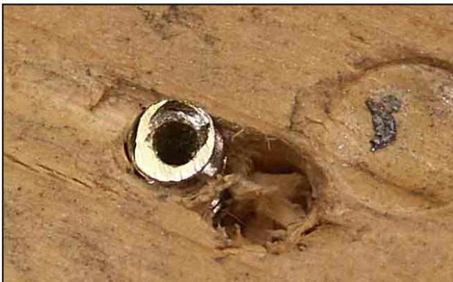
Fig 6—(above) To facilitate drilling a lengthwise hole in the #6-32 $\times\frac{3}{4}$  screw, drive it snugly into a  $\frac{3}{4}$ -inch-thick board. Here we see the drilled end of the screw slightly protruding from the board.
