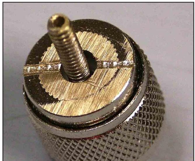
over them. Don't worry if the threads are not perfect on one end; just be sure that the end with the damaged threads goes on the PL-259 center pin when that step of assembly is reached.
