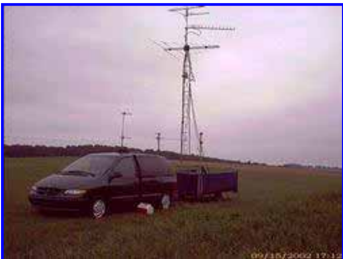
KF8QL/R and K8DOG set up in EN72. Log Ant. for 6/2/220, smYagi for 432, Loopers for 903/1296
