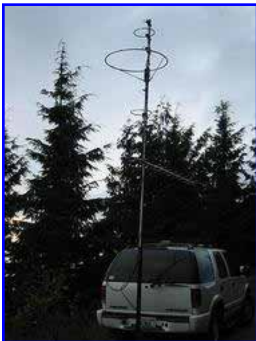
Stacked KB6KQ loops on 2M and 432, single on 6M. 21 element M2 432 yagi (2/3rds shown) proved a little too sharp for hand pointing and quick QSOs. Mast travels at 13ft. and easily pushes up to 17ft.
