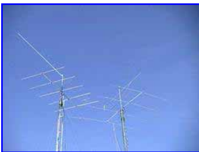
N7CZ North (rear) 3219 for 2M, K1FO for 70cm. South Tower (foreground) 222-5WL for 135cm, and A50-5S for 6M.
