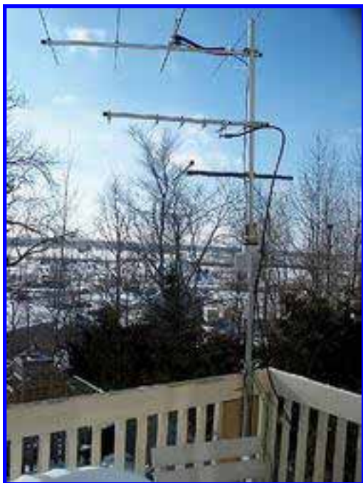
My limited antenna setup.. Cushcraft 4 ele for 144, 6 ele yagi for 432 (broken.. used a verticle instead) and a homebrew dipole for 220.
