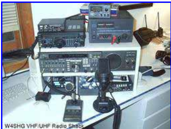
W4SHG Shack - Yaesu 847 and Yaesu 736 with MD-1 and MD-200 Microphones
