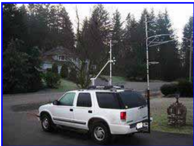
K7MDL Rover Rig on the launch pad in CN87. Stacked KB6KQ loops on 2M and 432, single KB6KQ loops on 6M and 222. Stacked homebrew 1296 big wheels under the 222 loop. 13ft. total height, 17ft. raised.
