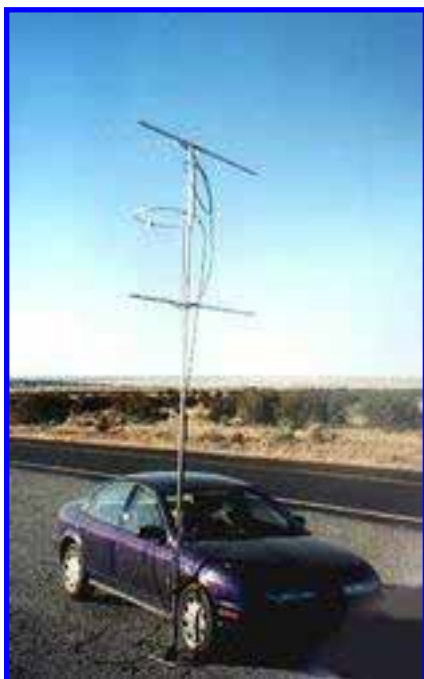
Running 170 Watts to stacked 5-el beams on 2-m; 100 Watts to a KB6KQ loop on 6-m.
