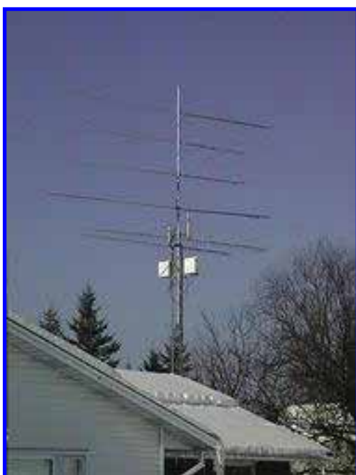
The Tower, Top to bottom - 432 30ele, 6mtr 5 ele, 222 16ele, 2mtr 14 ele, 903 47 ele, 1296 55ele, left box houses 903 & 1296 transverters, right box houses 432 and 222 transverters.
