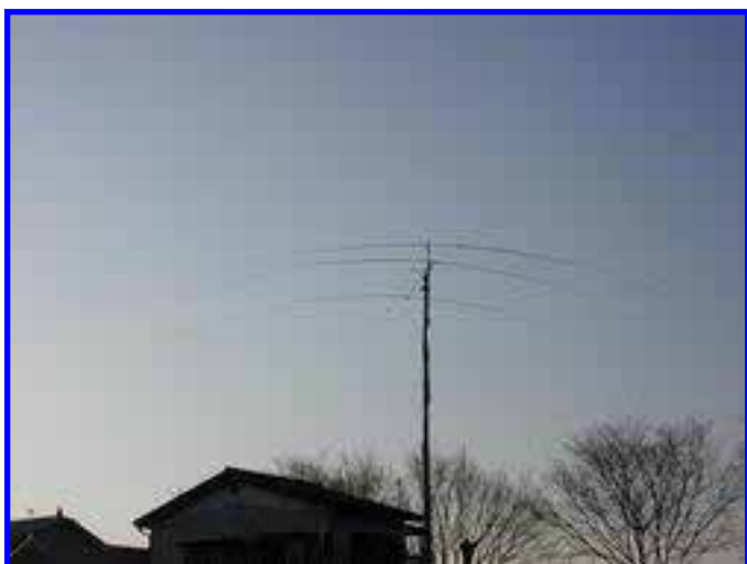
My new 3el full size yagi for 40m. de JH1AEP Fumi
