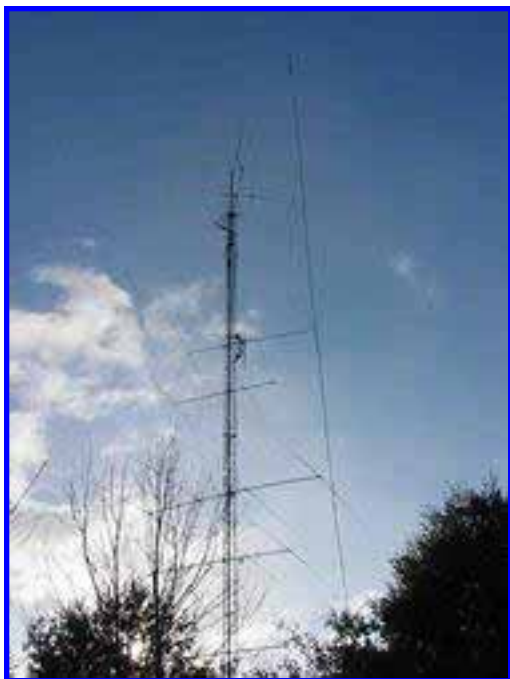
The main tower. Inv-V on 160 and 80, 2 el 40, 4/4 on each of 20, 15, and 10.
