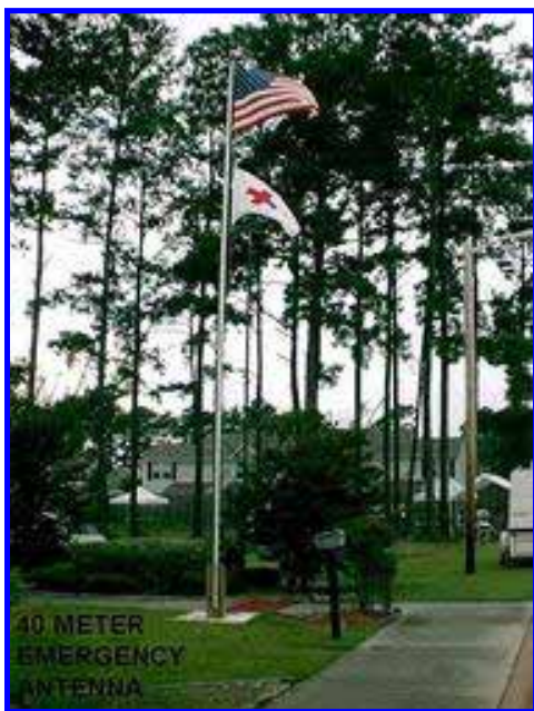
W4GS 40M Flagpole (Emergency) Antenna
