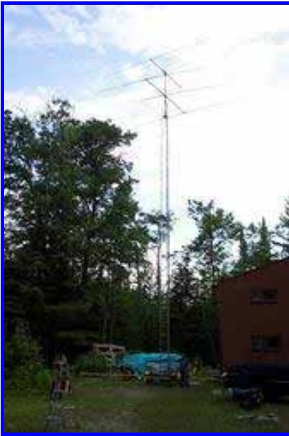
56' aluminum tower on N8KLX-designed trailer
