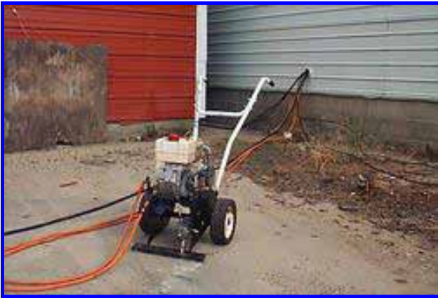
Home Made 12V generator. 5HP & Delco one wire generator kicks out 75 Amps at 13.8V.
