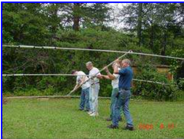
Assembling the A3S tribander.
