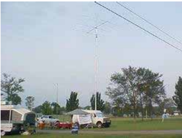
The K4MHK self-contained, fully-equipped, climate-controlled, mobile emergency communications vehicle complete with 40' pneumatic mast, rotor and 4-element yagi.
