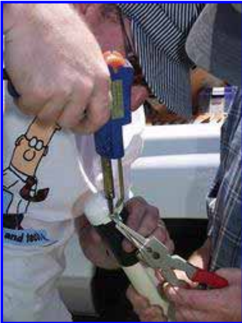
Soldering the 1:1 Balun
