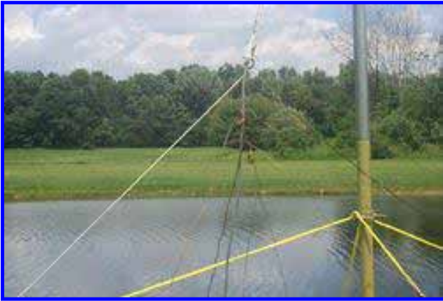
The 40M vertical feedpoint and radial connection (yes it worked!)
