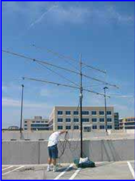
AA5AM (Scott) with the final touches on the VHF stack (6, 2, 70cm)
