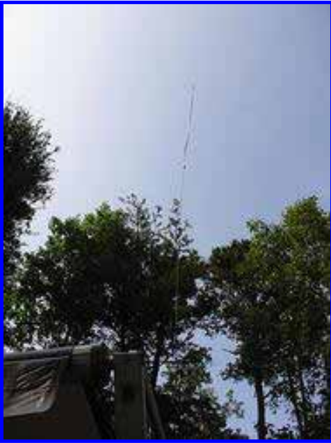
G5RV antenna shot up about 50' into the trees with my trusty antenna.
