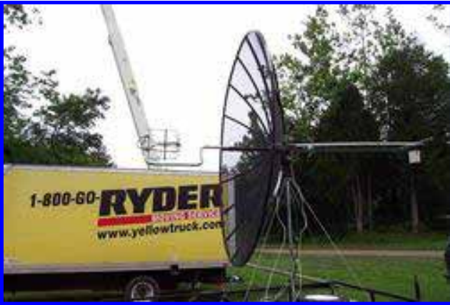
W4SHG AO-40 3.1 Meter Satellite Dish with the W0LMD Tri-Band Patch Feed. What a thrill to drag this through town on a trailer.
