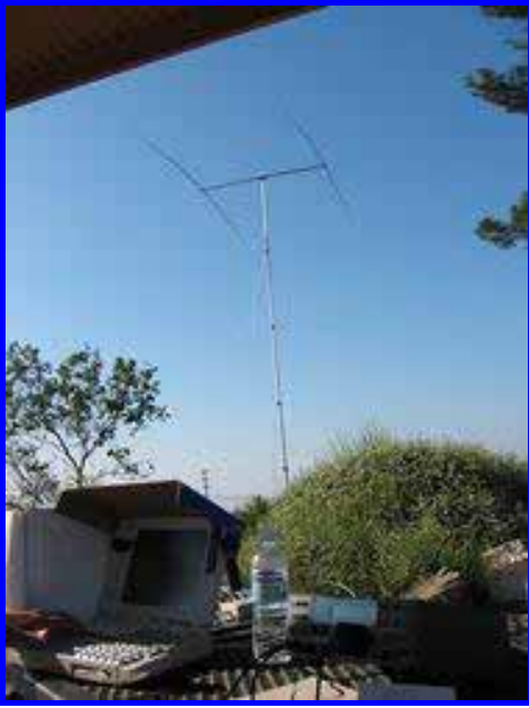
Superantenna's 2 ele Yagi shown set up for 20Mon 20 ft pushup mast.
