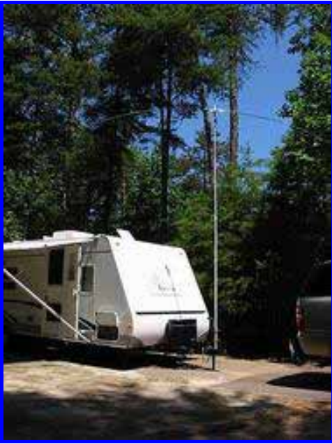
Hamstick dipole on an extendable swimming pool pole, u-bolted to the trailer jack.
