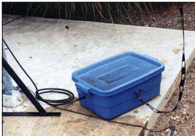
View of the 450- \Omega ladder line feeding the driven loop. The box on the pad is the transmatch described in the text.
