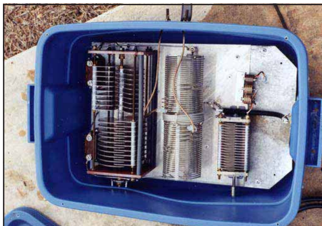
View of the interior of the transmatch box showing the components.
