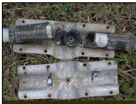
Serious TH7 bracket corrosion and insulator rot.
