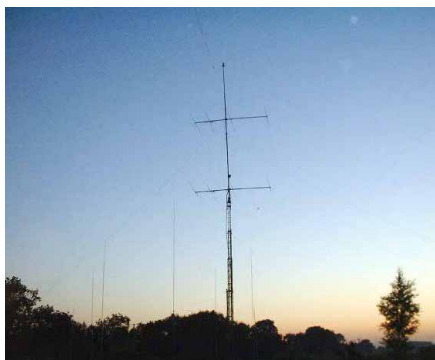
Ten meter four over four stack at G3LZQ's station. Dipole for 80 meters also used by GB5HQ and supported at the top of the mast extension.
