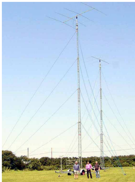
Pair of 15 meter 4 element yagis at 75 feet erected just for the contest at G3TXF's contest station in Devon. L to R Nigel, G3TXF, Ian, G3WVG and Roger, G3SXW.
