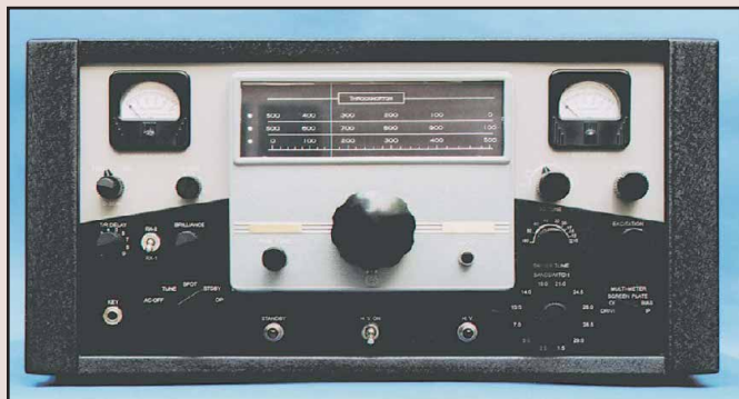
A new vintage transmitter: James Buchanan (JeRB), K8WPI, of Kalamazoo, Michigan, spent two years just digging for parts for his "new" transmitter, inspired by the T-9er from early 1970s ARRL Handbooks. The entire project took four years. JeRB writes: "The unit features a Vackar VFO offering linear tuning of 500 kHz band spread on 12 bands, all current and planned HF amateur bands. A 'vintage' transmitter that can hold its own in today's crowded bands and against receivers with 250 Hz filters places unique requirements on stability and frequency agility. It is now my primary transmitter. A matching antenna tuner and 12, 17 and 30-meter converter for use with a vintage receiver complete the station. It is a hoot!"
