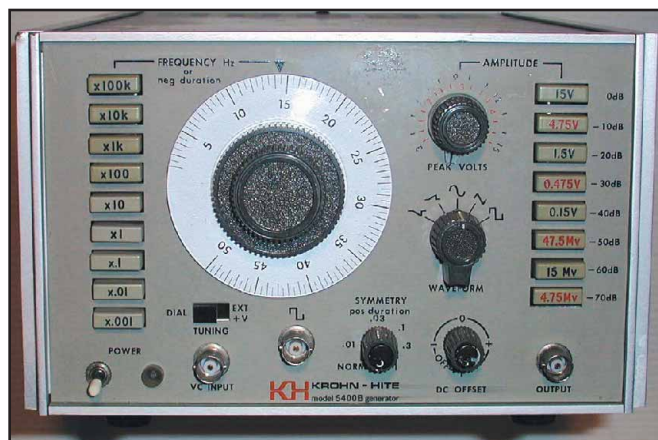
Figure 4—A basic function generator.
