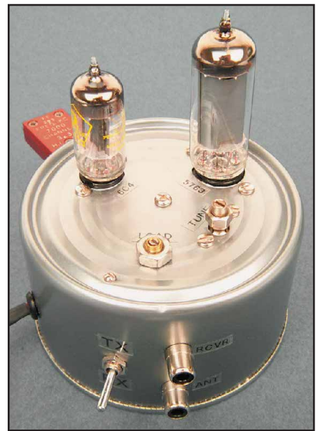
Figure 3B—A top view, showing the tube socket and plate tuning and loading capacitor layout.
