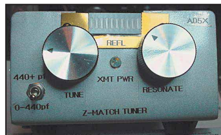
Figure 6—The bar graph display of reflected power makes tuning easier and more intuitive.
