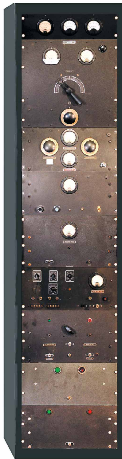
All the black front panel parts from the last station were placed in the 6 foot 6 inch cabinet for this photo. K2WI intends to try to rebuild this rig as close to original, as the present condition of the various units will permit. Most units have been modified over the years.
