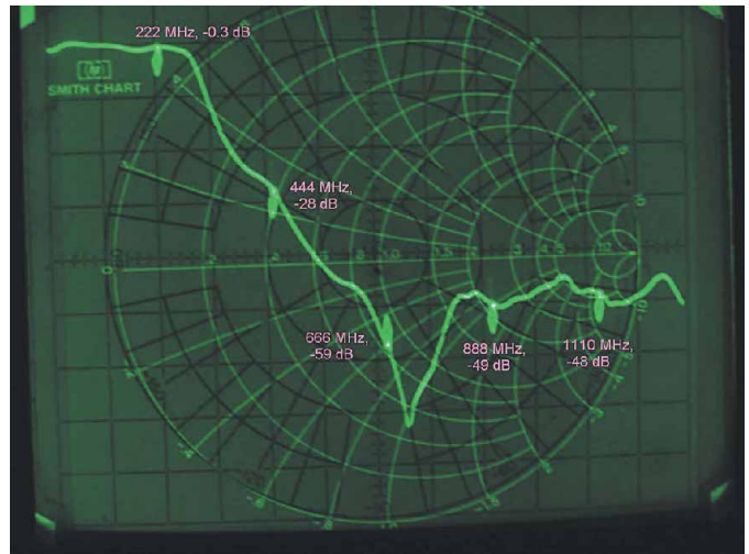
Figure 5—The output low-pass filter response.
