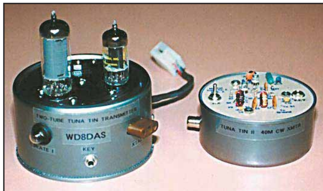
Figure 2—A side-by-side comparison: The T5 is on the left and the classic W1FB design, the Tuna Tin 2, is on the right
