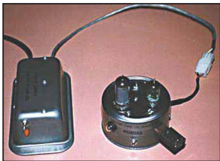
Figure 5—The completed project: Mini-Loaf power supply next to the T5.
