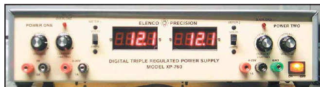
Figure 3—A variable multi-output power supply.
