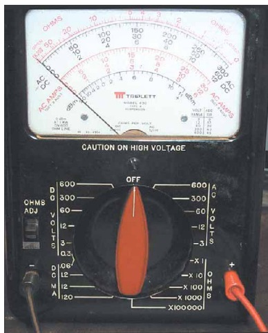
Figure 5—A typical analog type VOM.
