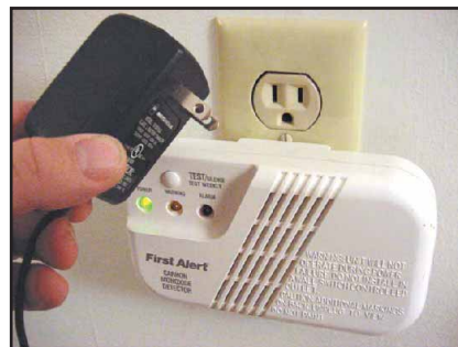
Figure 5—A smart wall-wart charger may falsely trigger a CO detector when they're on the same outlet.
