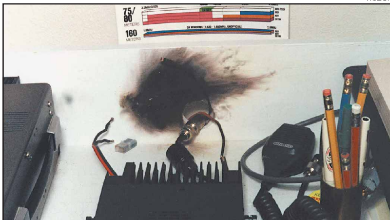
When a sudden, powerful bolt of lightning struck his house, Andrew Flower, W0ZUX, was admittedly not prepared. The result is the damage apparent in the photo—and there was more, both in the shack and outside. He had disconnected the coax from his gear, but there were no outdoor disconnects on his rotator cables. There are now...
