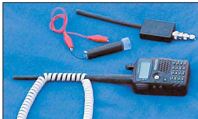
Figure 4—Several ways to boost the HF reception of general-coverage handheld radios with small flexible antennas.
