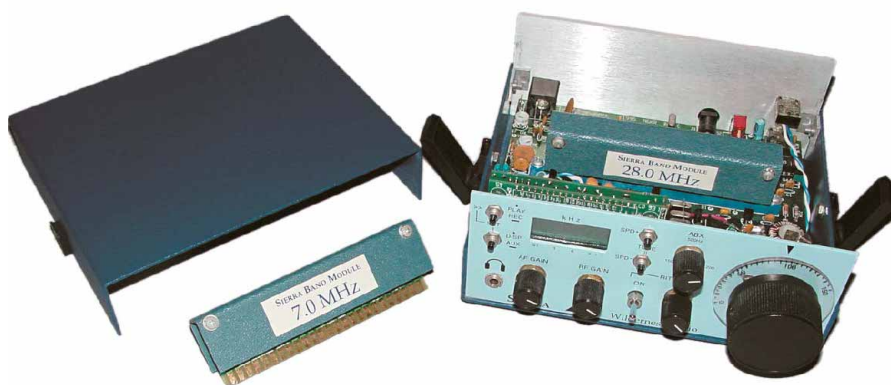
This photo shows one band module installed inside the rig. The Sierra features the KC-2 memory keyer/audio VFO module installed. The LCD display shows operating frequency, S-meter and RF power output.
