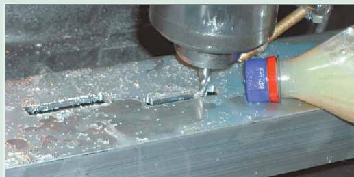
Figure A—The design of the slot antenna allows it to be easily reproduced with a milling machine.
