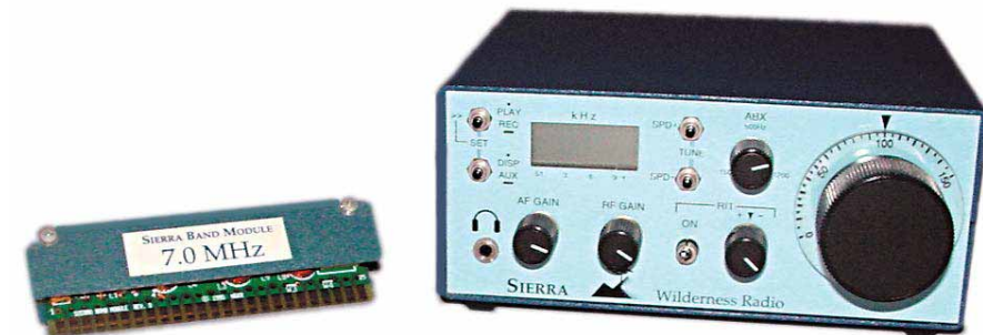
A view of the Wilderness Radio Sierra multi-band QRP CW transceiver pictured with one of its band modules. You can add as many modules to cover the bands you need to work.
