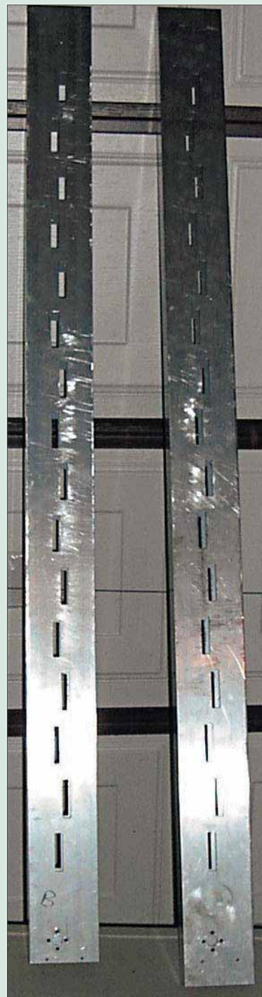
Figure B—Two freshly machined prototype slot antennas ready for finishing.
