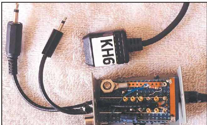
Figure 2—Each wire in the VC-H1 cable terminates in a gold-plated pin. The 11 pins provide versatility. I can easily reconfigure the pin connections if I change radios. The solder lug at the upper left provides a ground connection between the case and the ground bus on the perforated board.
