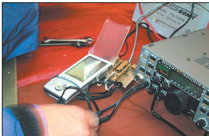
Our gear: Zaurus palmtop, NorCal paddle and Elecraft K2 transceiver.
