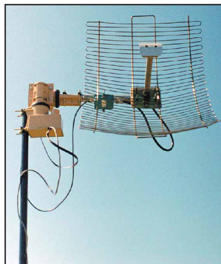
Figure 10—A single antenna mounted to one side. The rotator is ideal for positioning an S band antenna for receiving the AO-40 satellite.
