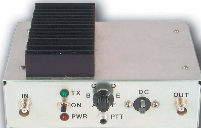
Figure 1—The completed 30 W amplifier. The band switch takes care of output low-pass filter switching.
