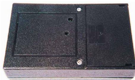
Figure 5—The rear panel of the MFJ-461. The 9-V battery compartment is at right. Within the rectangle at left, there are two screwdriver controls for audio frequency (top) and input level (center). The audio frequency setting is critical for proper operation.
