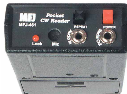
Figure 6—The side panel controls and jacks of the MFJ-461.
