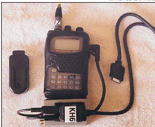
Figure 1—The VX-5R to VC-H1 setup. The interface box contains interconnecting jumpers that can change as equipment changes. The phone plugs increase versatility, enabling use with many transceivers.
