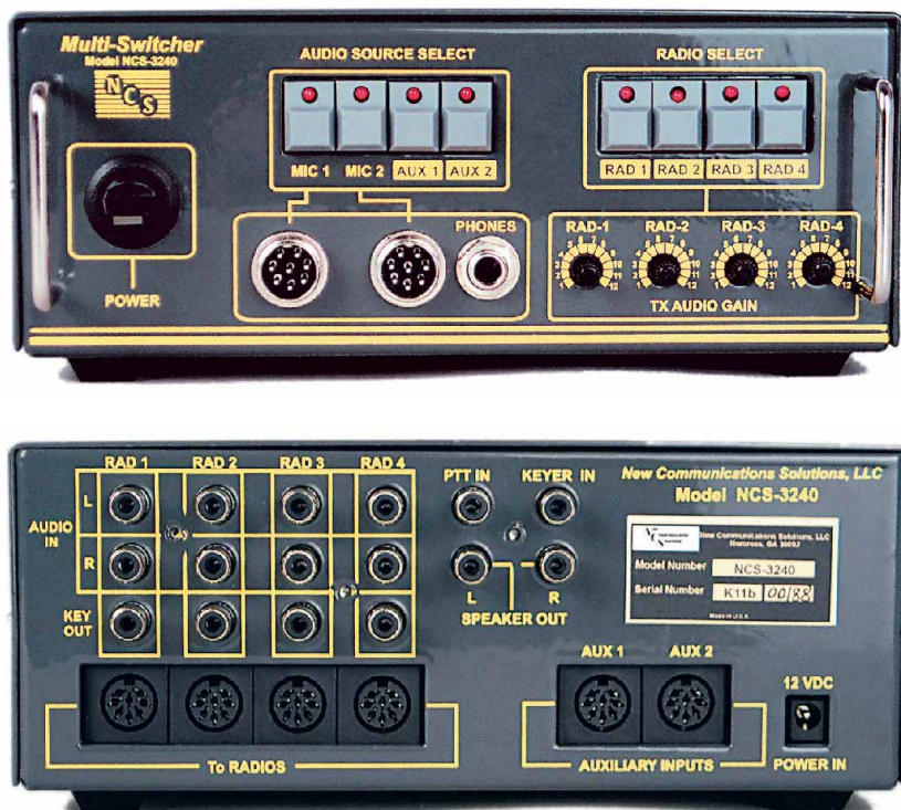
Figure 2—The rear panel of the NCS-3240.
