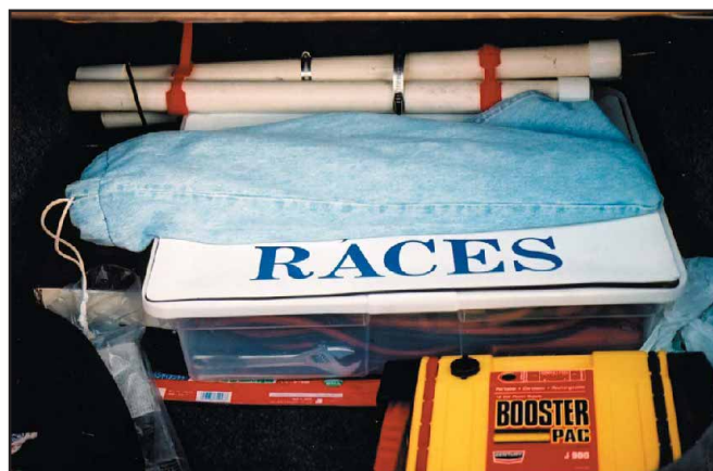
Figure 10—The car trunk includes a 12 V, 17 Ah gel cell, portable antennas, RF amplifier, leather gloves. The blue stuff sack on top of the bin stores a dual-band Yagi (Arrow OSCAR antenna).
