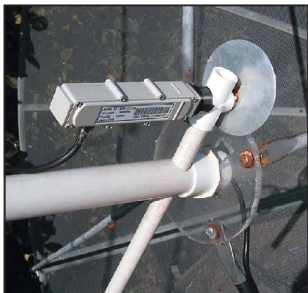
Figure 2—The offset feed patch feed support positioned above the dish. Note the radial arm support, which can be both rotated and offset from center to facilitate feed steering. The notch in the base plate for the N connector prime focus mount can be clearly seen. It is not used for the offset feed. The offset patch-type feed can be positioned to avoid being blocked by a strut.
