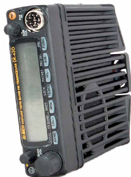
Figure 5—(Top) Is this a defect? Did Alinco manufacture this unit of the DR-620T upside down? No, not at all. Alinco allows the user to decide whether she wants the speaker facing up or facing down by rotating the front panel 180 degrees. (Right) As you can see, in this configuration, the speaker is at the bottom of the radio, ideal for mounting just under a shelf or dashboard.
