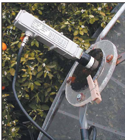
Figure 4—The prime focus feed mount showing the downconverter, adapter disk and the clothespin wedge for locking the prime focus adapter in place after it is centered.
