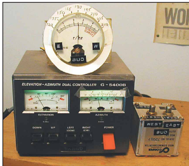
Figure 8—This azimuth indicator and switch box reveal their junk box origins. The Yaesu rotator control positions the uplink antenna. The meter is a surplus 75 μA movement, although other low current meters can be used.
