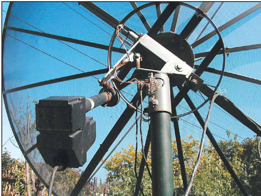
Figure 9—From left to right: actuator, actuator arm; polar angle adjustment; umbilical terminal wired to mount set screws, polar axis pivot bolt head and declination adjustment nut. The position-indicating potentiometer can be seen at top center, coupled to the polar axis bolt. Other than aligning the polar mount with Polaris (by sighting along the polar axis) no adjustments are made to polar or declination settings used for regular C band TV service.
