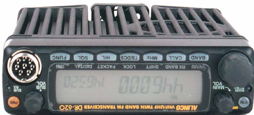
Figure 5—(Top) Is this a defect? Did Alinco manufacture this unit of the DR-620T upside down? No, not at all. Alinco allows the user to decide whether she wants the speaker facing up or facing down by rotating the front panel 180 degrees. (Right) As you can see, in this configuration, the speaker is at the bottom of the radio, ideal for mounting just under a shelf or dashboard.
