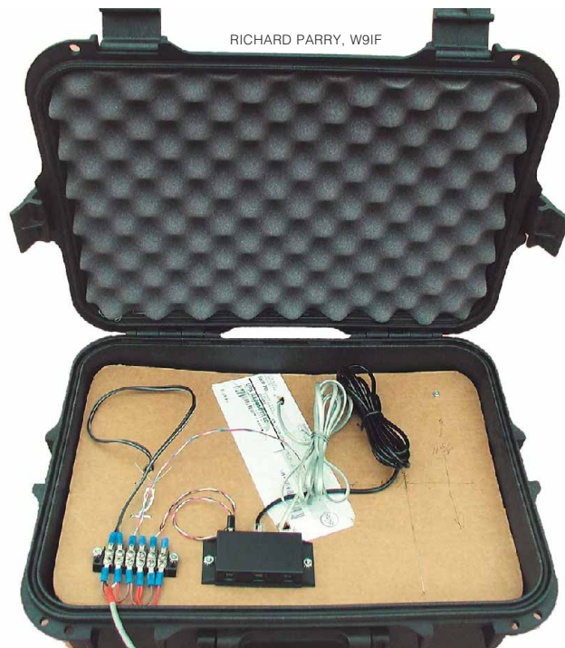
Figure 3—Bottom view of the APRS weather station. The terminal block provides for power distribution, while the junction box in bottom center interfaces the outdoor temperature sensor and anemometer.
