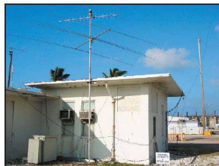
On 12 and 17 meters we used this four-element dual-bander by FinnFet Antenna.
