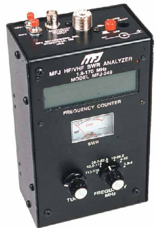
Figure 2—A portable antenna analyzer is a useful device for determining antenna and transmission line characteristics. It generates its own signal, so transmitter RF isn't required.
