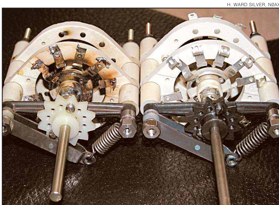
Figure 3—The band switch section on the left clearly shows the signs of destructive arcing.
