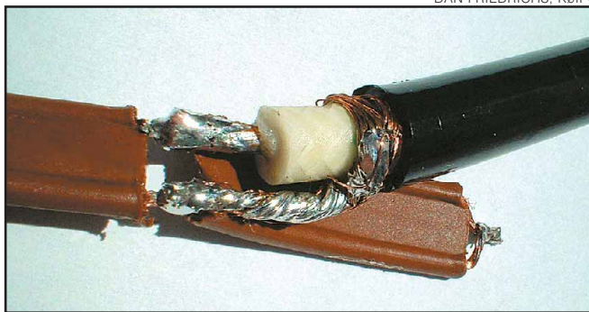
Figure 2—A look at the coaxial feed line, which is soldered to the bottom end of the matching section. The details are shown in Figure 1.
