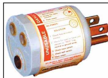
Figure 1—A simple electrical outlet tester can identify many local ac wiring problems.
