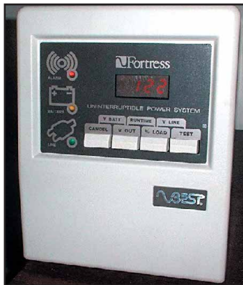
Figure 2—An Uninterruptible Power Supply (UPS) can correct for many line voltage level changes, spikes, line transients and outages. The better ones produce a sine waveform.
