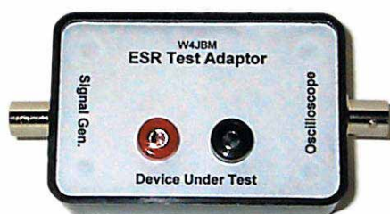
Figure 3—The ESR test adapter built by the author.
