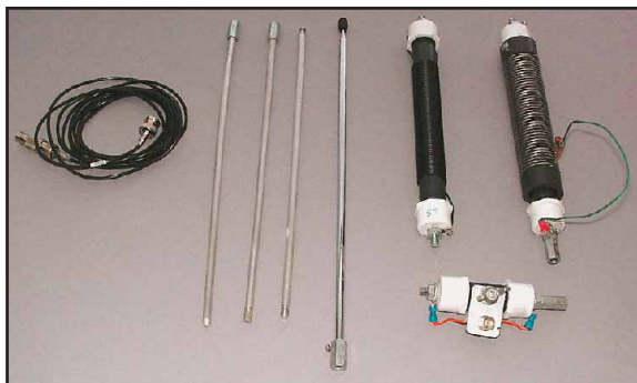
The entire PAC-12 antenna broken down for transport. The two coils in the photo are the 40 meter and 30-10 meter prototypes.
