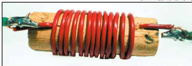
Figure 4—The decoupling coil is wound on a wooden dowel form. The radiating elements are then soldered to the coil.
