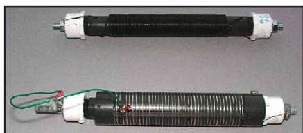
A close-up of the prototype multiband coil showing the shorting lead connected for operation on 30 meters.
