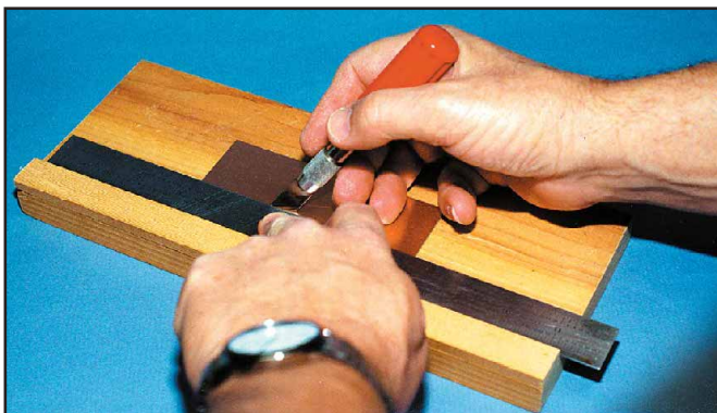
Figure 3—Keep everything snugly in place and against fixture dog, keep fingertips in back of the gauge edge, then score the material several times on both sides with a hobby knife.
