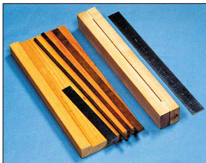
Figure 1—These are some of the simple fixture parts needed to build functional, good looking enclosures from printed-circuit material. A few dollars' worth of wood and metal are all that are needed.
