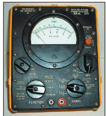
Figure 4—The front of the ME-418/PSM-37. To the right of the meter face are the OVERLOAD flag and the red RESET button. Below the meter are the OHMS adjustment (left) and the Polarity Switch—power OFF, +DC, -DC and AC (right). At the bottom right is the RANGE switch and bottom left is the FUNCTION switch.
