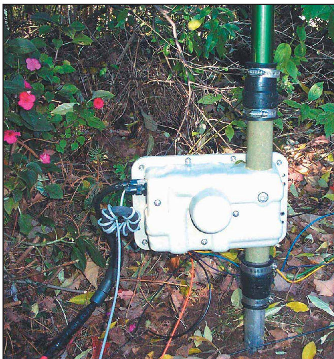
Figure 2—The SmallIR motor housing. You'll notice the chokes I installed on the control cable and feed line to minimize common-mode currents.
