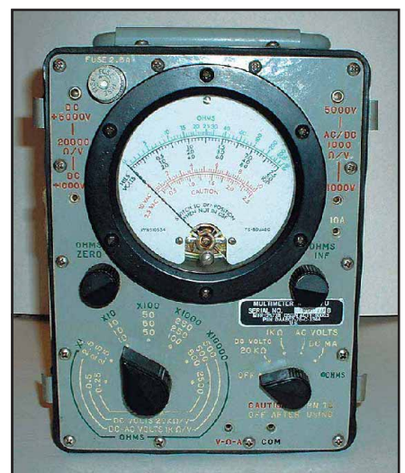
Figure 3—The ME-297/U. The line fuse is at the top left. The round knobs are OHMS ZERO (left) and OHMS INF (right). The range switch is to the left and the function switch to the right. A removable cover (not shown) contains the test leads.
