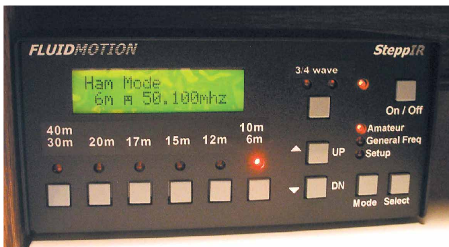
Figure 4—The SteppIR controller is compact at only 6 inches in length. In this view, you see it sitting atop my station computer (the crinkled appearance of the display was caused by the fact that I hadn't yet removed the protective plastic film). All of the antenna tuning is accomplished here.
