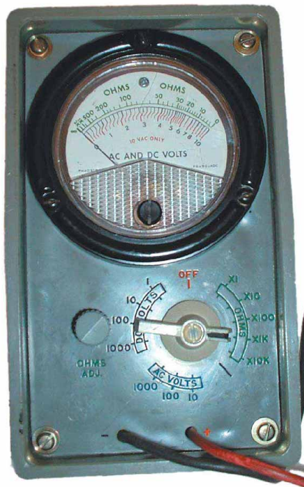
Figure 2—The ME-77/U with the cover open. The range switch is to the right. The round knob to the left is the ohmmeter adjustment. Notice that the test leads are integral to the meter and cannot be detached.
