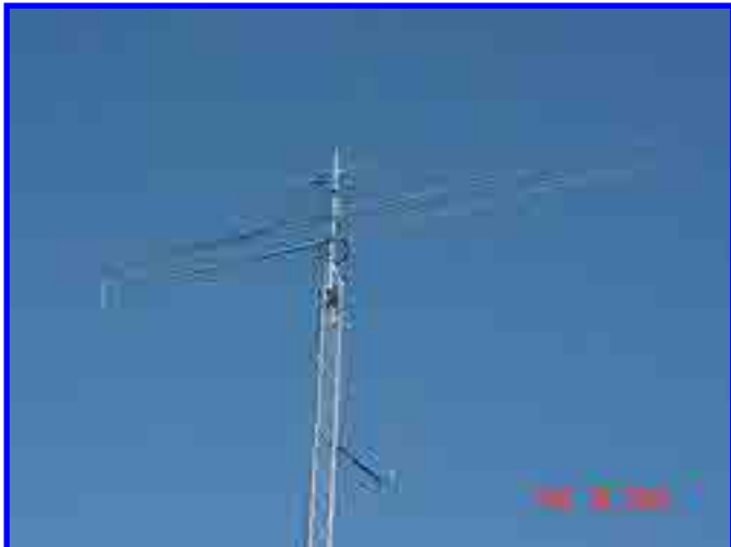
Top to bottom: 3 elt 6m, 10 elt 222, M2 432-13WL, Cushcraft 4218XL. 2m J-Pole at lower right is my APRS IGATE station.
