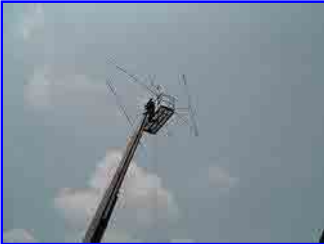
A tri-bander, a 40-meter rotatable dipole, and 3 wire antennas on a 60-foot man lift provided many options for contacts on different bands through the entire contest.
