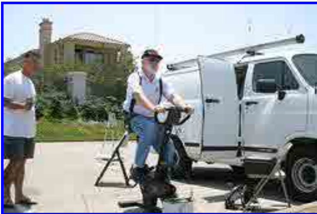
Peter, AD6TN built this Human Powered Battery Charger. Tim, WD6AWP, urges him on to see that voltage is high enough to charge the battery pack. Get a good cardiovascular workout, and generate power at the same time! We weren't able to calculate how many VPG (volts per Gatoraide) but it was an interesting source of power. . . .
