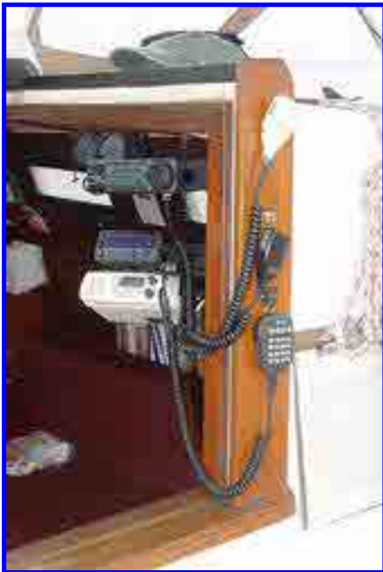
Top: HF operating station, ICOM 706mkII Middle: VHF/UHF station, Kenwood TM-V7A Lower: VHF marine radio
