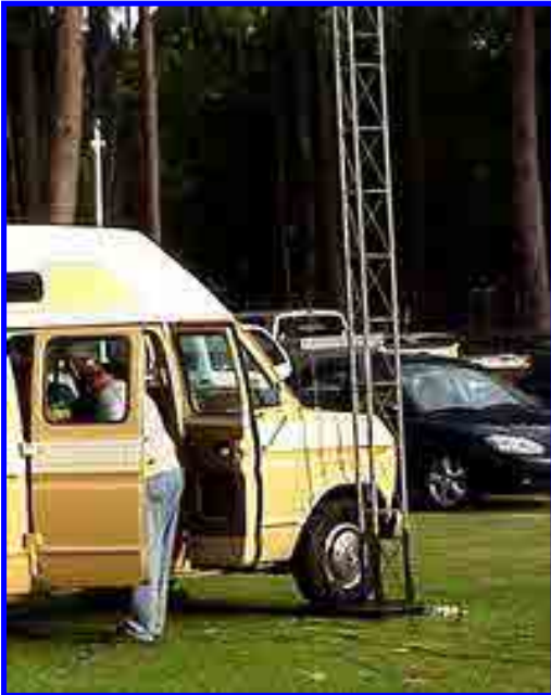
The tower mechanism is of Mac, KF4GLE's design. It utilizes a hinged tower base, anchored by the passenger side wheel. A second platform, anchored by the driver side wheel, holds a pole with an electric winch, for raising/lowering the tower.
