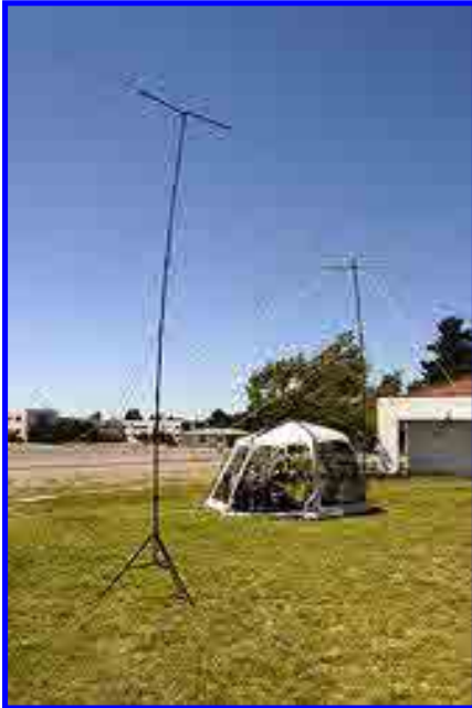
Operations tent with 10/15 Meter Buddiepole and 20 Meter Yagi.
