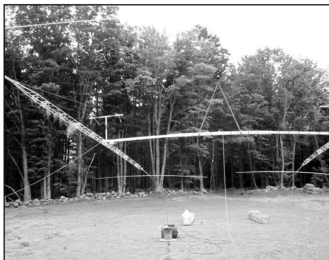
Figure 2—Tuning the Force 12 2 element 80 meter Yagi.
