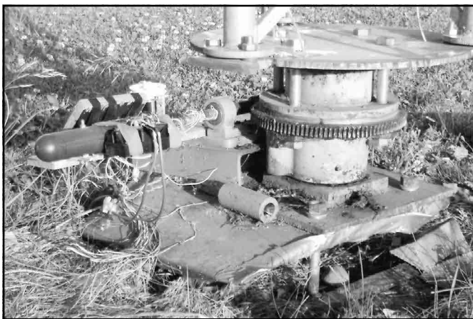
Figure 2—Shown is the rotor for a small rotating tower at OH6LI's home. The 3.3 v battery operated screwdriver motor is turning an angle transmission found in a junkyard. The original use of the angle transmission was likely some paper mill equipment. The tower is in a suburban area and is 24 meters tall with a 2 element 40 meter and a five band Yagi, all of which are easily rotated with this system.
