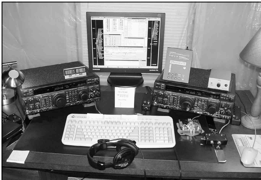
A typical SO2R station layout. Is everything located to optimize performance and minimize fatigue?
