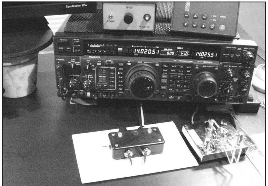
Figure 1—The home-brew SO2R audio controller at N4GG. Audio CW sidetone has been replaced by a keyed LED.
