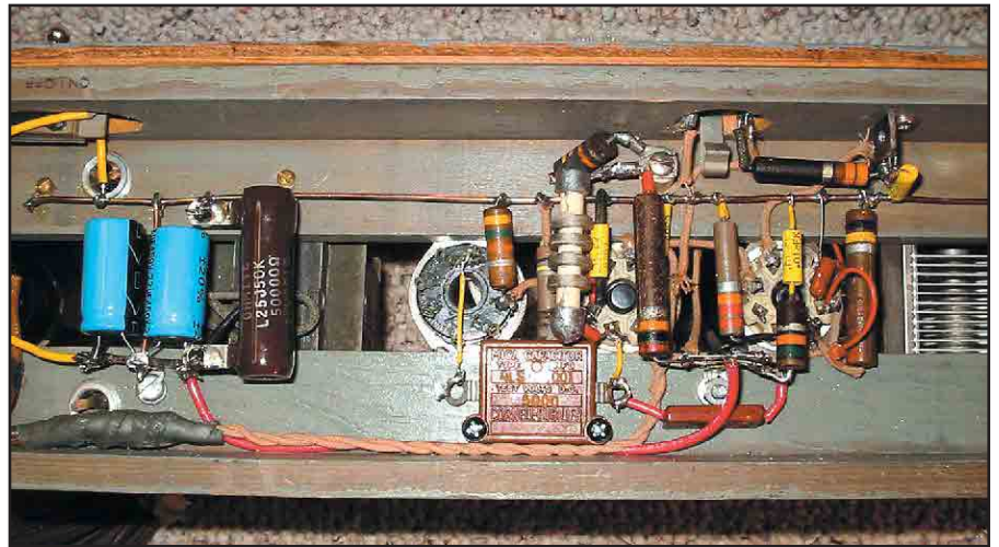
Figure 4—A close-up of the below-chassis wiring. Transmitter wiring closely follows the original 1948 article in The Radio Amateur's Handbook .
