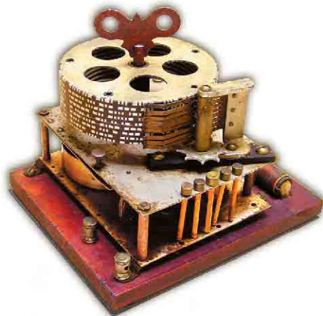
Figure 5—The Natrometer, a commercial version of the Omnigraph.
