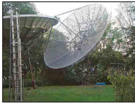
Figure 2—At right, the well known 8.5 meter Kennedy dish at K2UYH. At left, a new 4 meter dish for 10 GHz.
