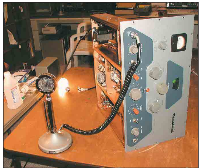
Figure 8—The finished DX-100 delivering power to a load. It's great to see that bulb lit by RF.
