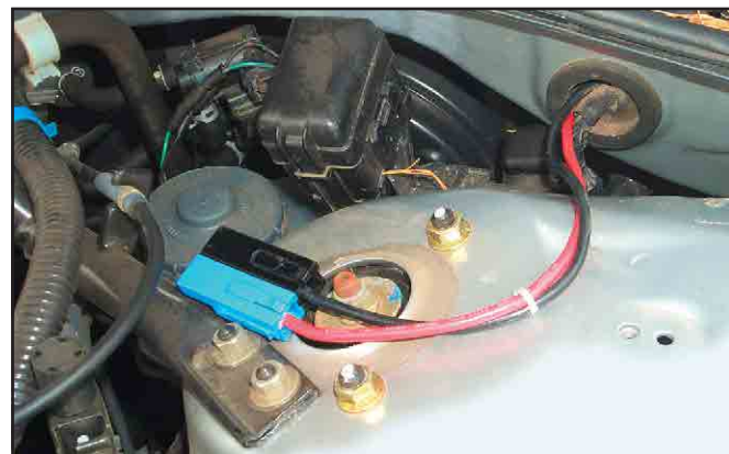
Figure 1—An example of a dc power cable firewall grommet installation. Note the high current connectors. These will make it easier to route the remainder of the line to the battery terminals.
