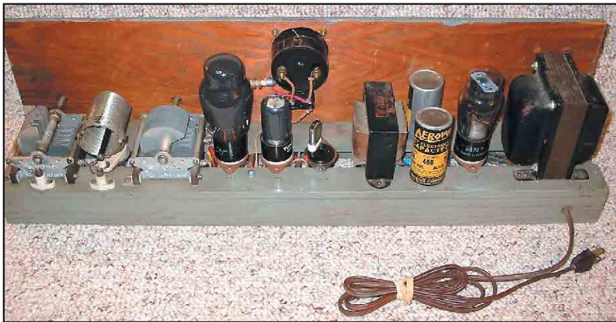
Figure 2—A rear view of the restored transmitter. Note that the power supply is common to the transmitter chassis.
