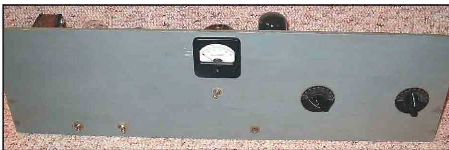
Figure 3—The front panel. The milliammeter, key jack and power supply switches were modifications by the original builder.
