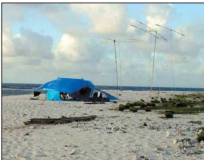
Figure 4—The Serbian base sported two beams, a vertical and two inverted Vs for the low bands.
