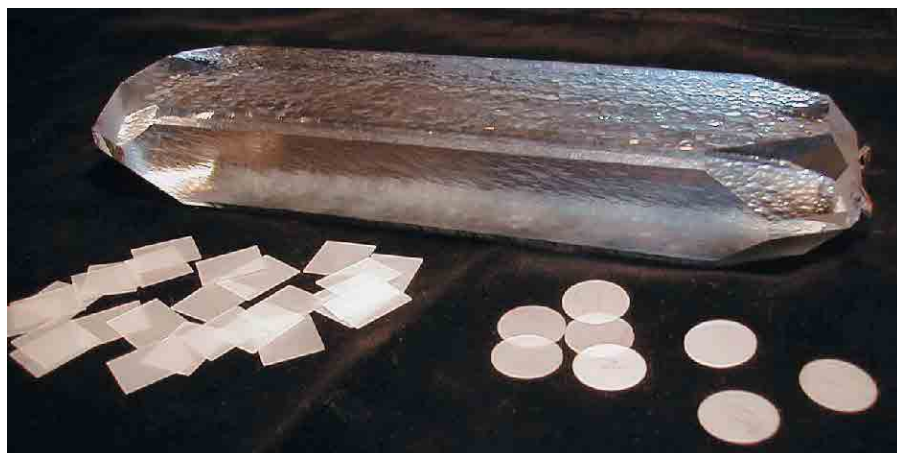
Figure 1—A bar of cultured quartz alongside examples of the types of wafers that might be sawed from it. (The bar is 20.5 cm long and 2.5 cm thick; the blanks are only 0.35 mm thick.)
