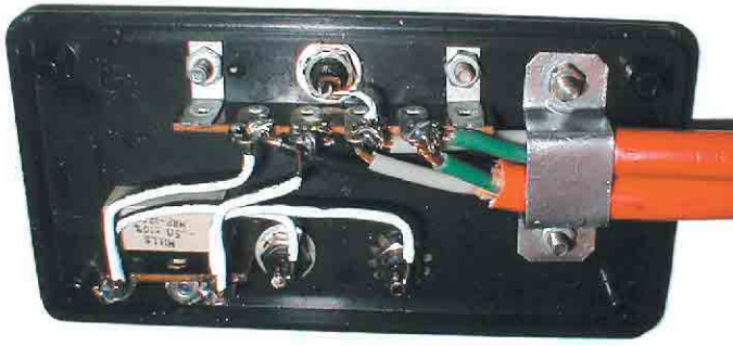
Figure 3—Wattmeter parts mounting on the enclosure panel. Note the current sampling resistor at the lower left of the panel.
