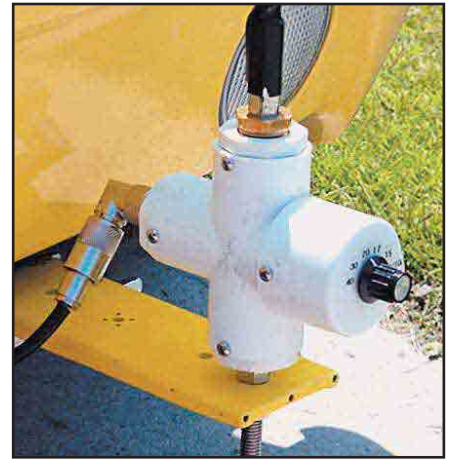
Figure 8—The completed assembly, consisting of mount, bracket, feed line and antenna, attached to the car and "ready to roll."
