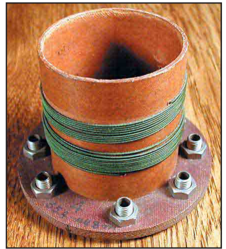
Figure 4—A close-up of a detector coil.
