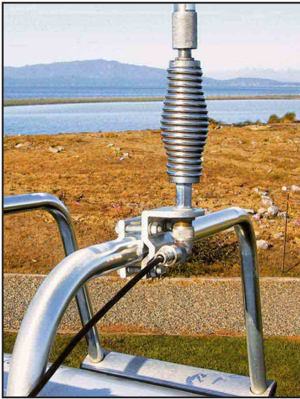
Figure 1 —On rental RVs, the ladder is about the only place strong enough to hold an HF antenna. Simple mounts often prove to be the most effective. After installing it, make sure you stop after a few miles and recheck all your hardware for tightness.
