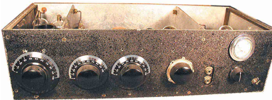
Figure 1—A front view of the Fred Schnell regenerative receiver. The meter measures filament voltage—a useful feature for battery-operated sets.
