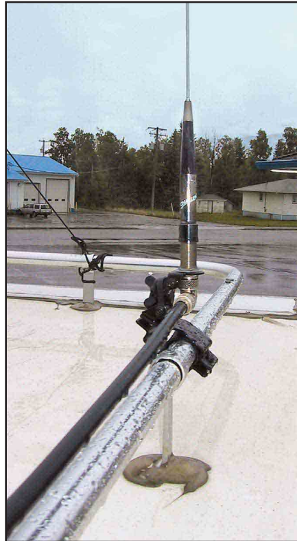
Figure 2 —For strong, easy, non-destructive temporary installations of lightweight VHF/UHF antennas on RV ladders or fragile railings, it's hard to beat today's "pipe clamp" mounts.
