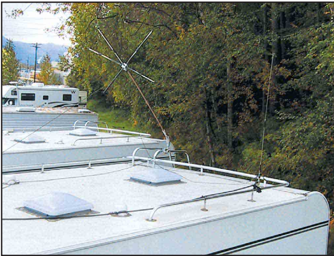
Figure 4—My finished RV antenna installation demonstrates my frighteningly simple overhead obstacle avoidance system: Pull your antenna over until it's low enough and mark your fore-aft guy rope with tape. As you approach a low-clearance point, pull in the guy until you see the tape. Works every time.
