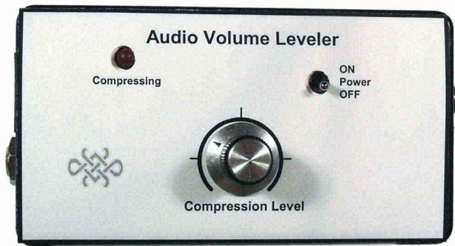
Figure 3—The front panel of the volume leveler. The “compressing” LED shows when leveling is taking place.
