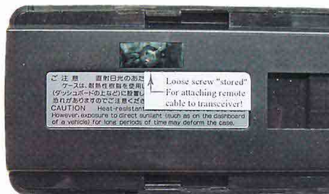
Figure 2—KO8S stores the cable retaining screw for his ICOM's remote front panel kit in a recess on the back of the panel.
