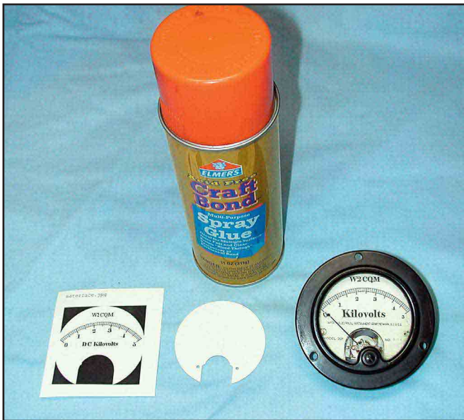
Figure 1—Two candidates for meter scaling. Note the new meter face, the painted meter mounting panel (white) and the newly scaled meter face affixed with the spray adhesive.
