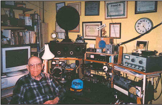
Creative indoor antenna: A ham for 65 years, Paul Fritsch, W3HHC, of Allentown, Pennsylvania, uses what he describes as a “very oddball antenna.” He writes: “The dark strip on the right of the photo goes up the wall to the ceiling, left and left again. It is a 16 foot piece of conducting wrapper from a steak sandwich. I also use the air conditioning metal ductwork as an antenna and have worked DX with both. Removal of all outside antennas was made necessary when I had the house sided.” There’s more on indoor antennas in the article that begins on page 28.
