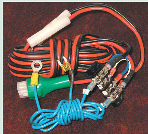
Figure A —The entire rental car power interface consists of the transceiver's 6 foot modular cable connected through a terminal strip to about 3 feet of 12 gauge lead wire. Extra terminals are jumpered and available to power accessories like my DSP-assisted external speaker.
