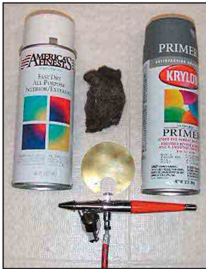
Figure 3—A view of the simple supplies needed to prepare the meter plate for the new scale. Spray-can white, primer and some fine steel wool. The airbrush is an alternative. The meter backing plate has been cleaned and ready for the new face.
