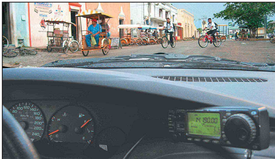
Figure 1—As we passed through outlying towns south of Mérida, Yucatán's capital city, DX signals abounded, bringing an "at home" operating environment to the rental car, despite the exotic surroundings. The separated control panel of the '706 enabled me to tuck it into an easily accessible spot where I could safely operate and drive at the same time.
