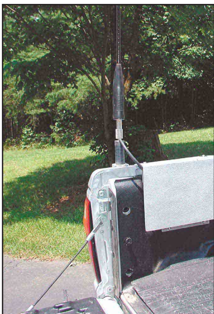
Figure 3—The tuner installation showing the homebrew Kydex protective cover in place.
