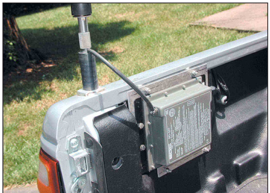
Figure 2—SG-237 antenna tuner mounted inside the pickup truck bed, showing the antenna base and the homebrew Delrin insulator.
