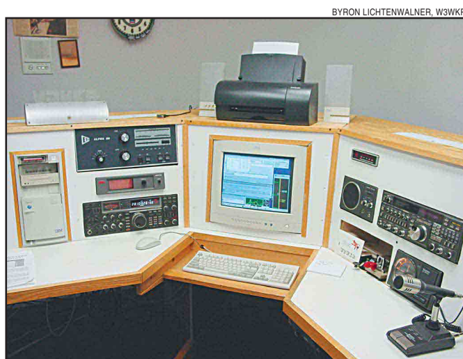
Byron Lichtenwalner, W3WKR, of Stroudsburg, Pennsylvania, searches the bands from this impressive station. It features an ICOM IC-765, PK900 TNC, Alpha amplifier, IBM PC running Writelog and a Mosley PRO-57B at 65 feet on a crankup tower.
