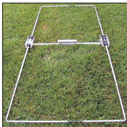
Figure 2—A bottom view of the completed antenna clearly shows the fiberglass insulators separating the driven element from the reflector.
