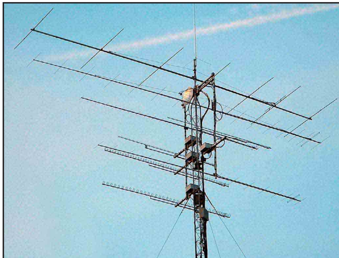
Figure 1—The N1DPM antenna stack in FN32. Notice how Fred tower-mounts transverters for his 903, 1296, 2304 and 3456 MHz and his 10 GHz 2 foot dish. Notice also that all antennas and gear can be serviced by climbing on the tower, without removing anything else to reach it.
