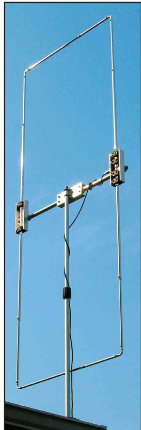
Figure 9—The Moxon mounted for vertical polarization.
