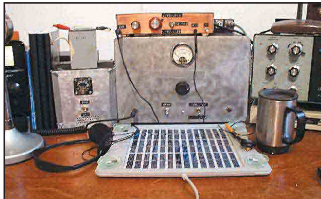
Figure 3—The 17 meter SSB rig again, this time in the Azores. The small box to the left is a linear amp (which takes it to 20 W PEP) based on a Ramsey kit. The solar panel is of the type being supplied with new Volkswagens—I use it to top off my gel cell (even here in London!). The copper colored box is my homebrew 20 meter DSB portable rig.
