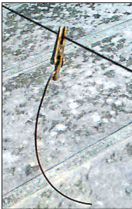
Figure 1—Temporary attachment of capacitance wires to the antenna using an alligator clip.
