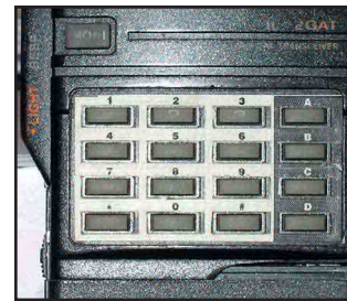
Figure 5—N2ERN repairs a whole keypad with well-placed cutouts.
