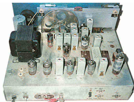
The SX-146 covers all frequencies between 2 and 30 MHz with an external oscillator, with the exception of the rig's intermediate frequency of 9 MHz.
