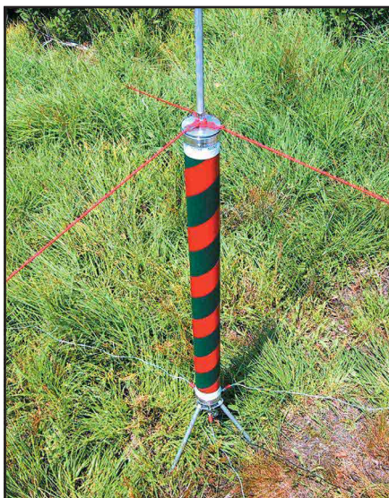
Figure 11—Close view of the FRV guy and ground wires. The ground consists of six 24 gauge, 20 foot wires attached to the VP-1 with alligator clips (two ground wires per clip).
