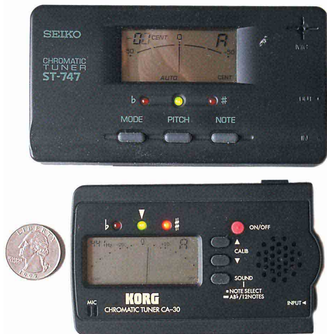
Figure 1—Musical instrument tuners like these can help the CW operator quickly and accurately tune a transmitter to the frequency of another station.
