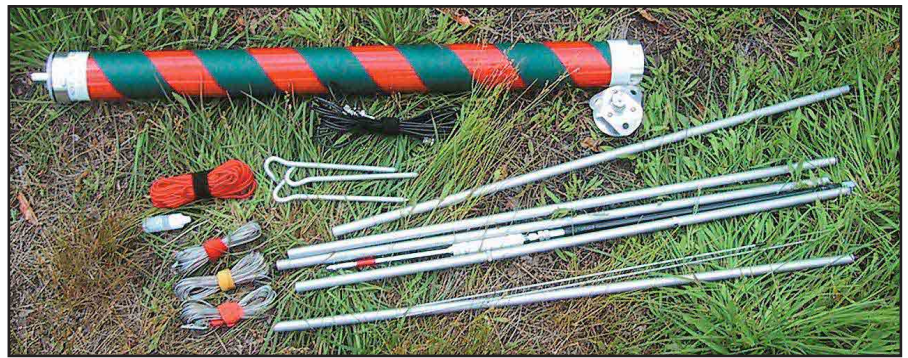
Figure 13—The disassembled Fly Rod Vertical. If you use a fat 2 1/2 inch diameter fly rod tube, you can stuff it all in, including the feed line.
