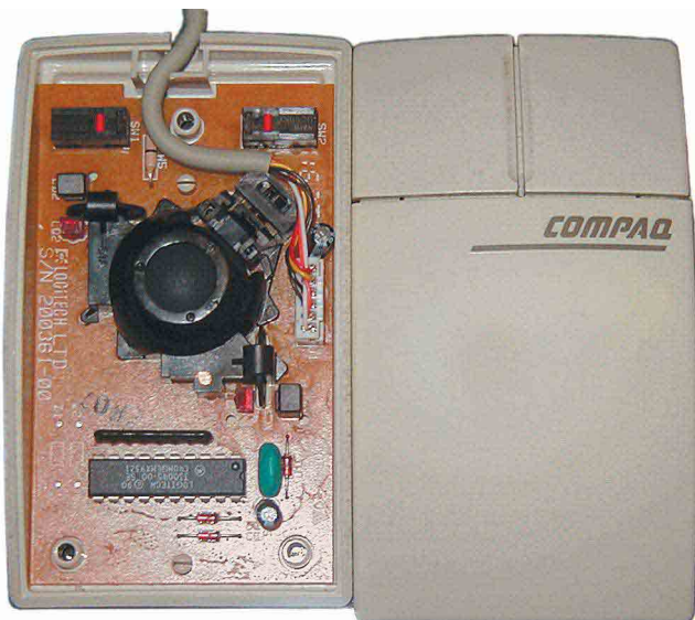
Figure 2—The mouse uncovered. Most of these components will be removed.
