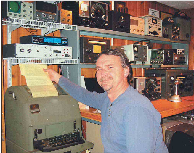
Here is a vintage RTTY station still being used today. It belongs to Scott Freeberg, WA9WFA. Just above the Model 15 Teletype is his vintage solid-state HAL ST-6 Demodulator. He also uses the Heath Monitor Scope for tuning in the RTTY signal. Scott's first experience with Teletype was back in the early 1970s aboard the USS Okinawa , sitting off the coast of Vietnam. Later, in college, he learned about ham radio RTTY and has been active since.
