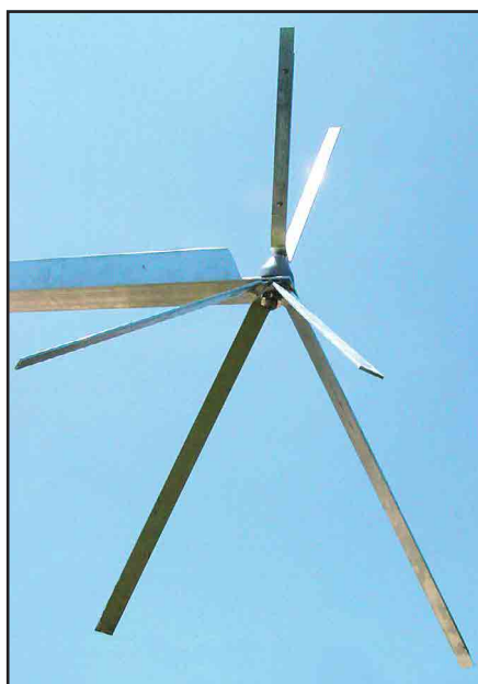
Figure 1—The side-mounted broadband tri-band VHF-UHF ground-plane antenna is made of aluminum flat-stock.
