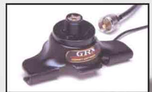
COMET GRB-5M Trunk lip mount, low-profile, black anodized stainless steel. Offset washers provide up to 17 deg vertical adjustment of antenna. 16'9" of deluxe cable included, 18" of mini RG-188A/U style coax for easy entry thru the weather seal. Gold-plated SO-239/PL-259 connectors.
