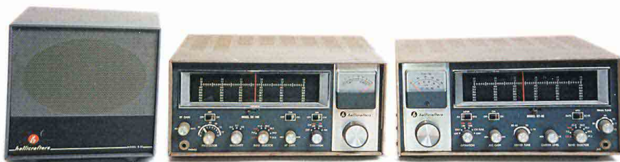
The SX-146 and HT-46 can be coupled together to share a VFO for transceive operation.
