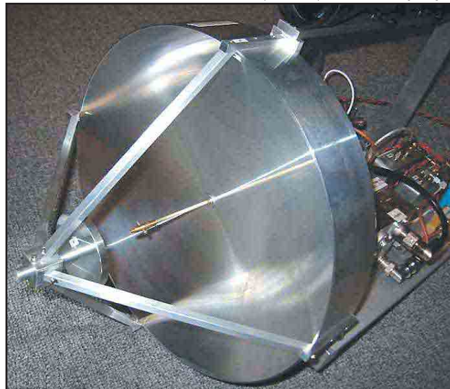
Figure 1—Homebrew 30 cm parabolic reflector with Cassegrain feed system used for the new 241 GHz record. The feed is a W2IMU-style dual-mode horn and the gain is estimated to be about 53 dB.
