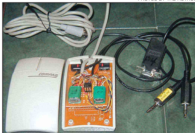
Figure 4—The completed mouse data/PC interface. The components mount to a sub-board that is then glued to the main board.
