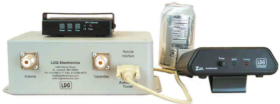
Figure 2—LDG RT-11 (left) with control box and Z-100. A 12 ounce beverage container is included for scale.
