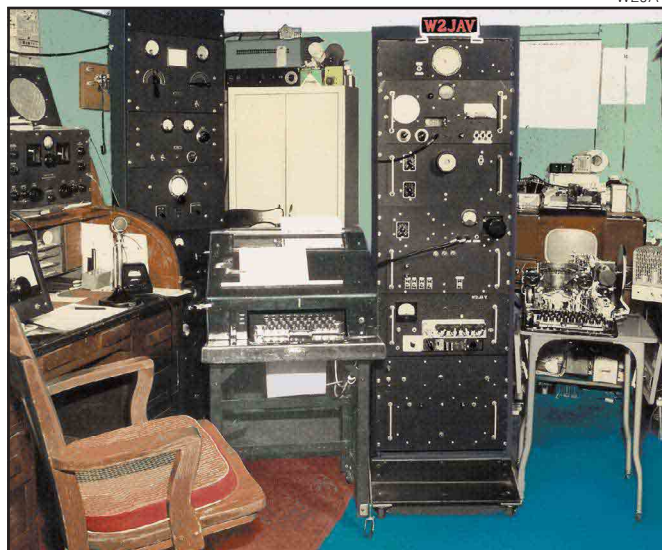
Phil Catona, W2JAV's, 1952 RTTY station in Hammonton, New Jersey. The large TTY in the center is a Teletype Model 12, and on the right with the cover removed is a Model 14. The relay rack with his call on top, contains all of the circuits needed for radio teletype. The other relay rack, left, is his homebrew transmitter. His Hammarlund Super-Pro receiver is on top of the desk.
