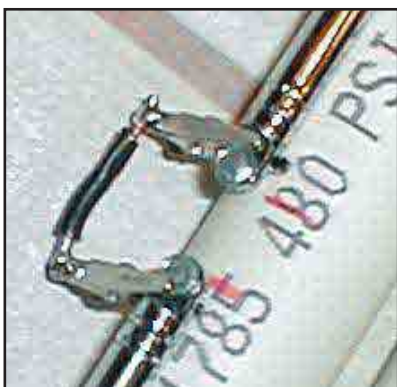
Figure 3—The shorting bar that enables the antenna to be used as a 12 foot vertical.
