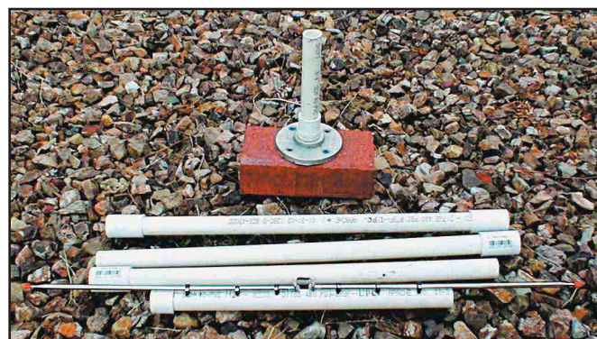
Figure 2 —The antenna breaks down easily for storage. Self-supporting and easy to set up, it weighs 8 pounds including base. No water flows through these pipes—only pure RF.
