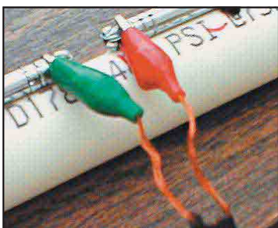
Figure 4—Close-up showing the connection that allows the Q&D antenna to be used as a center-fed dipole.
