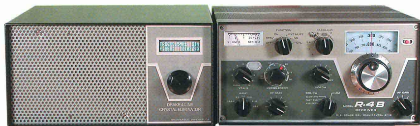
receivers shown alongside one of these popular receivers (an R-4B). The synthesizer allows any band within the receiver's frequency range to be tuned without crystals.
