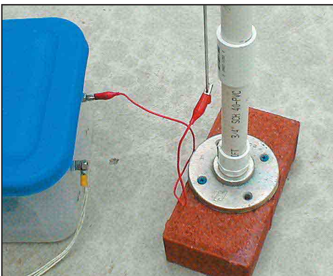
Figure 5—The base and connections to the tuner for operation as a vertical antenna.
