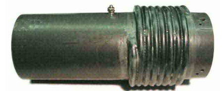
Figure 6—Completed 80 meter trap assembly ready to install.
