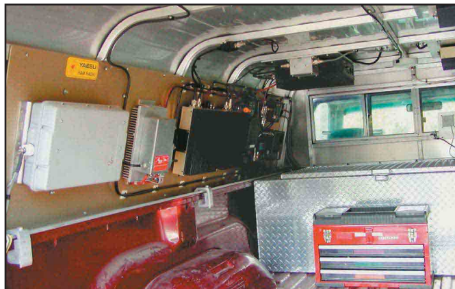
Figure 6—Under the cap. The business end of the K3CB rover showing 23 cm, 70 cm and 6 m amps to the left, a 2 m amp on the ceiling and a 222 MHz amp in the rear. Not shown are the two 1500 W inverters mounted on the right side.
