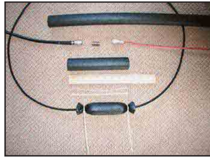
Figure 2 —A low-cost but effective way to waterproof cable connectors in the field. A short length of pipe insulation does the job.
