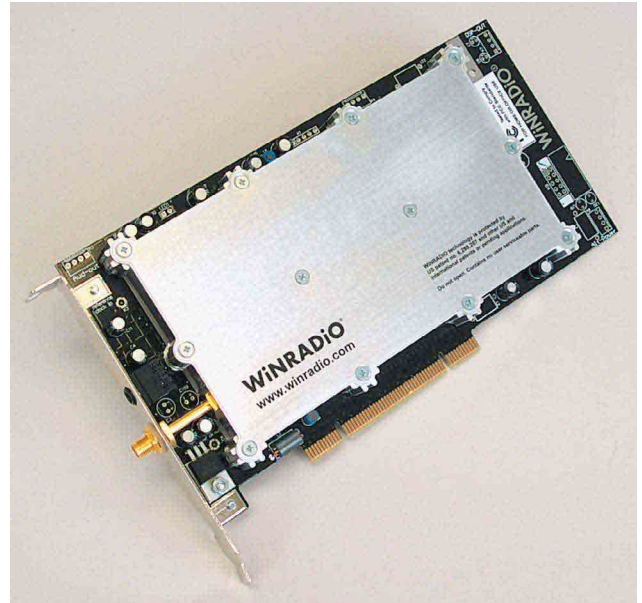
Figure 1—The top of the PCI card WiNRADiO G303i hardware.
