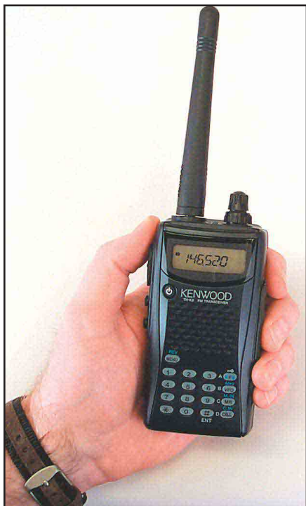
Figure 7—The TH-K2AT 2 meter transceiver is compact yet big enough not to get lost in your hand!
