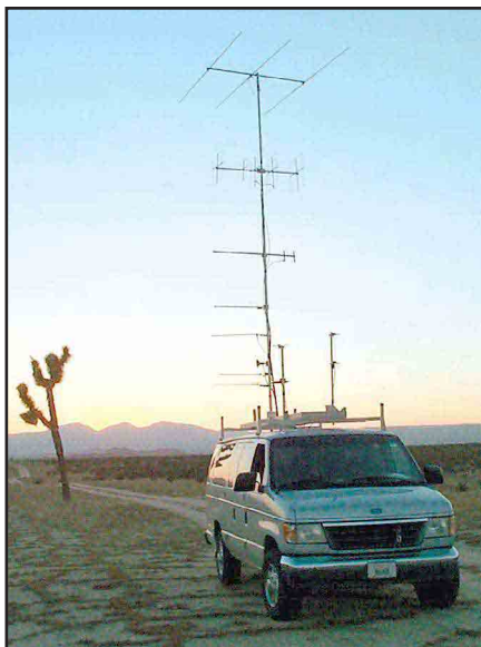
Figure 1—The N6NB rover wagon with antennas fully deployed.
