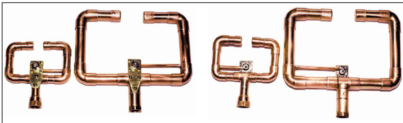
Figure 1—Front (left) and rear (right) views of the completed copper loops. The gamma tube penetrates the inner wall of the main element and is soldered parallel to the main lower tube. The connector mounting plate is anchored with self-tapping screws on the main and support tube centerline. The larger antenna is the 222 MHz version.
