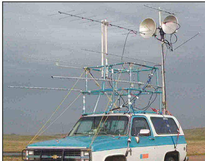
Figure 4—The N0DQS rover. Notice the PVC pipe mounts.
