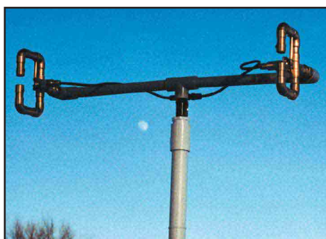
Figure 7— The complete loop antenna assembly shown in a stacked configuration for vertical-mode polarization.
