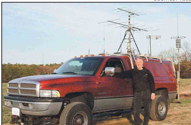
Figure 5—K3CB and the big red truck. Weak signal antennas are mounted on the tripod and a telescoping pole mounted off the right bumper.
