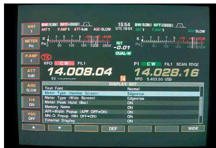
Figure 2—Selecting the edge-view metering for variety (no you can't have one of each!).
