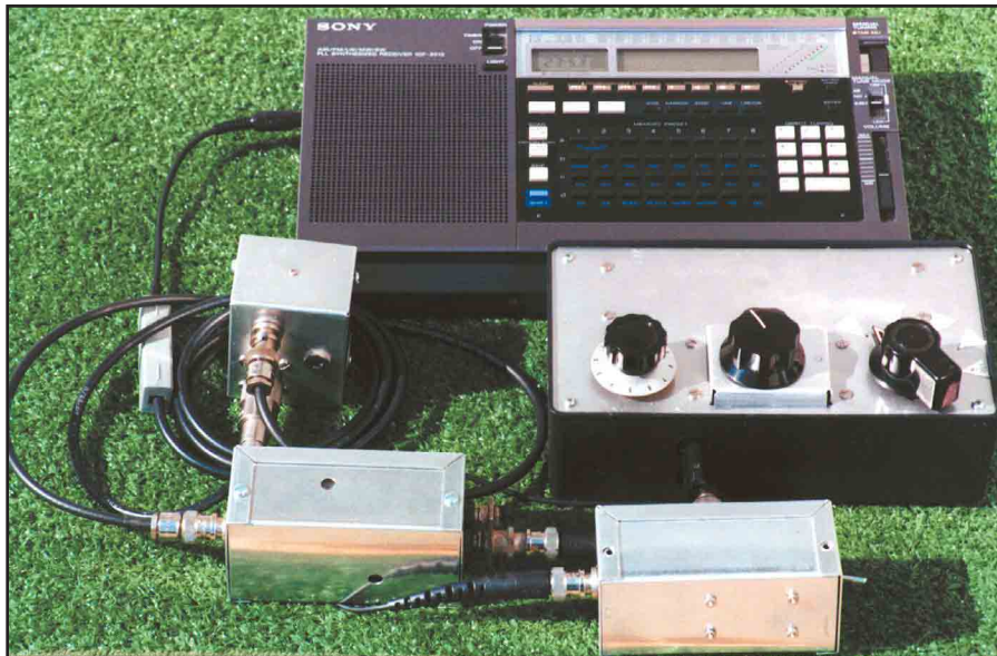
Figure 8—The complete LF receiving setup. The box below the antenna is a 20 dB high impedance preamplifier. The box to the left is the receiving upconverter. Above the converter is a power adapter for the upconverter. The converter and preamplifier are available from several suppliers (see text).
