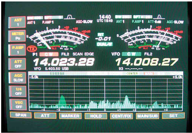
Figure 1—The normal IC-7800 display showing the emulated D'Arsonval meters above the spectrum scope.
