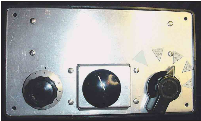
Figure 7—Front panel of the completed LF antenna. The coil selection switch is on the right, the tuning capacitor is in the center and the capacitor selector switch is to the left.
