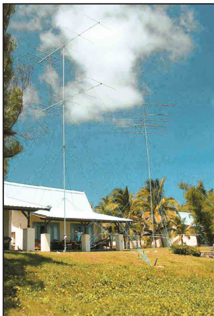
The 6-element, 10-meter Yagi and the 6-over-6 6-meter array, in front of the operating shacks.
