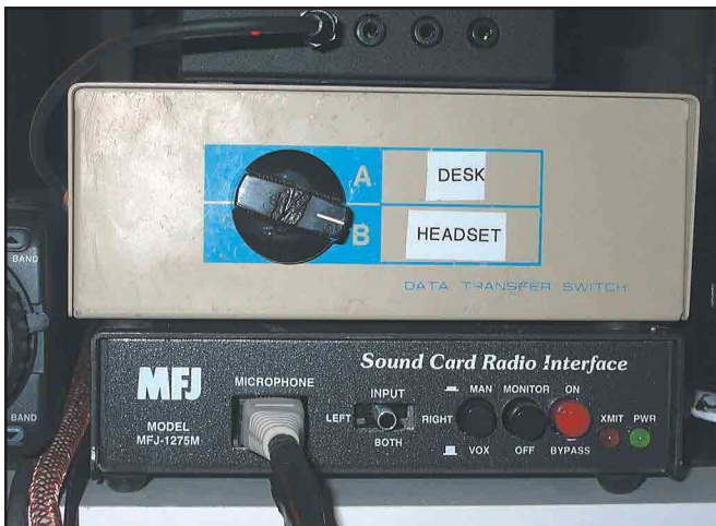
Figure 2—The data port switch configured as an A-B microphone switch. A front view.
