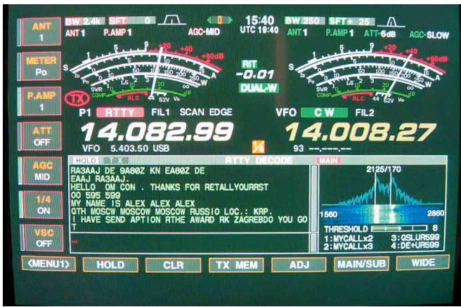
Figure 9—IC-7800 in RTTY mode, copying with internal decoder.
