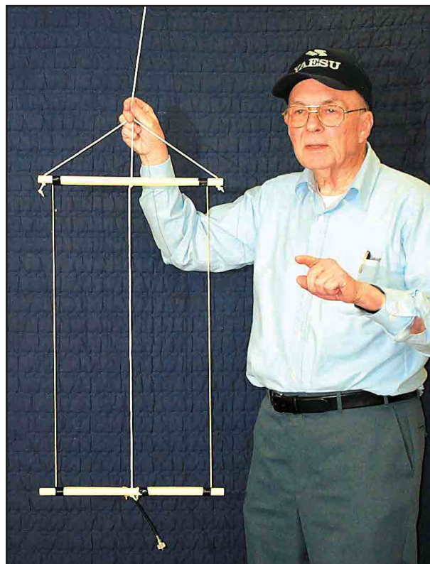
Figure 1 —At a radio club meeting, the author explains the hanging rectangular loop using a scale model of the antenna. The antenna shown is a workable 2 meter loop. Although the antenna has relatively low gain at VHF, the smaller model serves well to illustrate the design.
