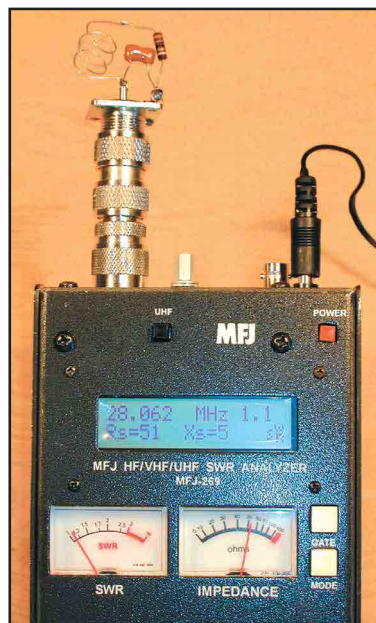
Figure 3—An SO-239 acts as a good prototyping platform for working with L-networks. An RF analyzer is shown and is convenient, although a low power transmitter and an SWR bridge will work.
