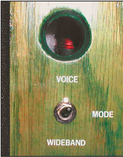
Figure 15—A closeup of the front panel switch labels and tuned port.
