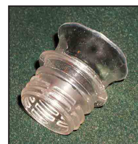
Figure 6—The flared port tube is made from the top of a plastic 2 liter soft drink bottle.
