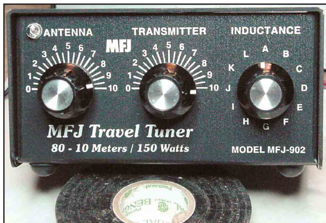
Figure 4—The modified front panel of the MFJ-902.
