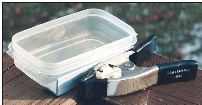
Figure 3 —The assembly configuration for the tower-mounted parts holder. Note the aluminum angle stock screwed to the clamp and the container.
