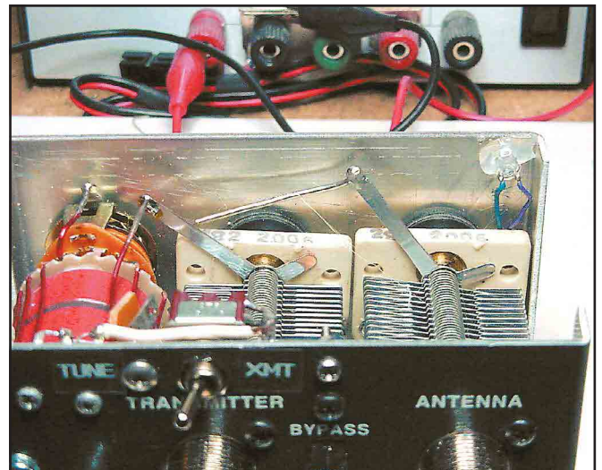
Figure 5—The LED attachment with hot-melt glue on the front panel (viewed from inside).
