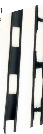
Figure 1 —The "stealthy" ladder line on the right can be made by cutting the line with "nail-slot-hole pliers" used for punching oblong holes in aluminum and vinyl siding. The line is then sprayed with non-carbon pigment foliage colored paint.
