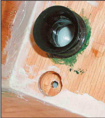
Figure 8 —The hole for the switch is recessed. Note the caulked interior. The enclosure must be airtight, including the back. This means that the front panel switch and rear panel input jack must also be sealed.
