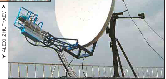
The 2.4 meter offset-fed dish at RW3BP used to hear the first lunar echoes on 47 GHz.
