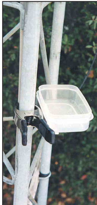
Figure 2 —The parts holder in use, mounted to a tower leg.
