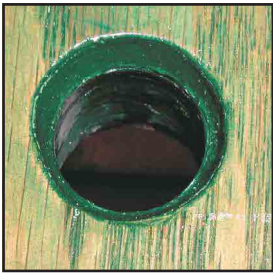
Figure 7 —The front of the tuned port is flared (tapered) slightly with putty as it doesn't fully extend to the surface of the front panel.
