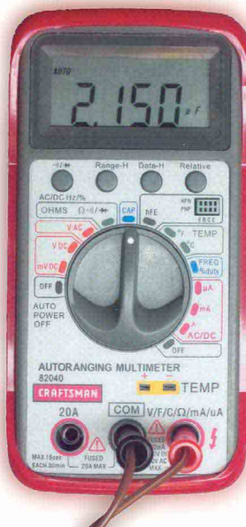
Figure 2—A typical autoranging DVM (Craftsman #82040) used with the SMD tweezers.
