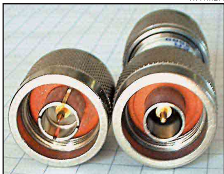
Figure 2—Male N connectors. On the left is a slotted, and on the right a higher performance slotless connector.
