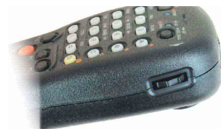
Figure 6—Tuning wheel on the side of the MH-59 Remote Control Microphone.
