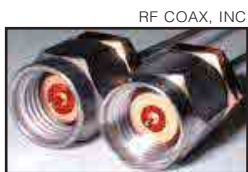
Figure 8—Here are a male 2.9 mm SMA compatible connector on left, and male 2.4 mm (not SMA compatible) connector on the right.
