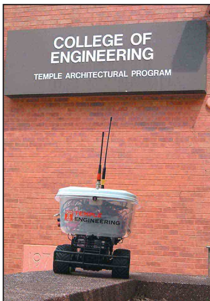
Figure 3—The TUARC Earth-bound Mars Rover outside and underway. The Rover has been controlled and the surroundings seen and heard over 5 miles away using the K3TU club station antennas.
