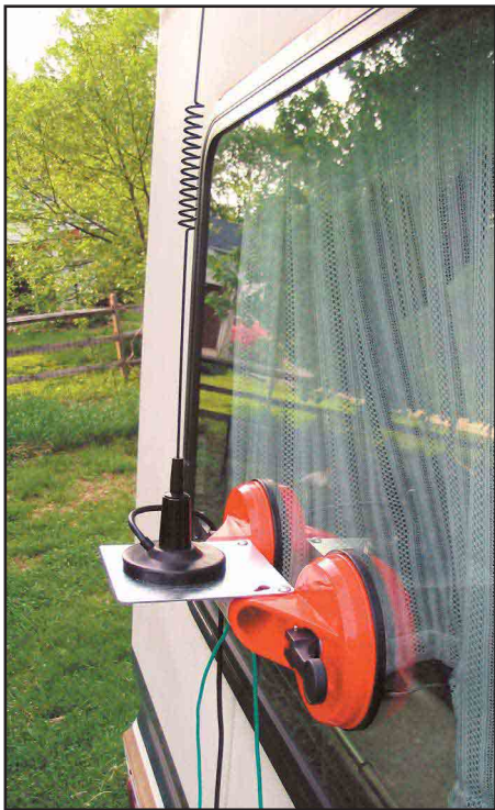
Figure 4—With metallic surfaces hard to come by on the bus, this mag mount assembly did the trick.
