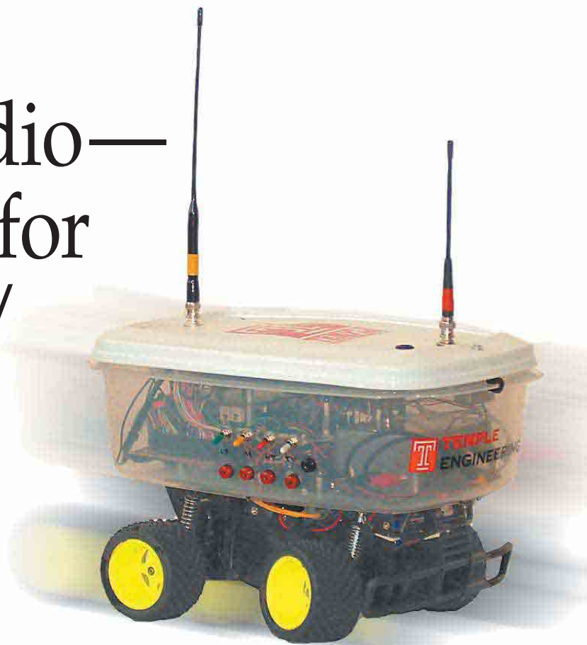
Figure 1—The completed TUARC Earth-bound Mars Rover. The ATV camera is mounted under the lid on the right side. The 2 m and 70 cm rubber whip antennas are mounted on a ground plane that is under the lid. The toggle switches and jacks are for control and monitoring of the battery subsystems.
