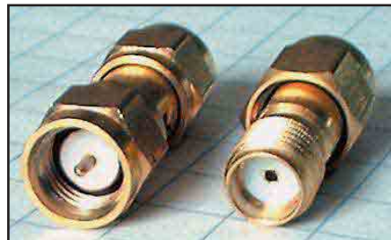
Figure 5—A pair of SMA connectors, with male on the left and female on the right. Like many connectors, these are available in nickel, stainless steel or gold finish.
