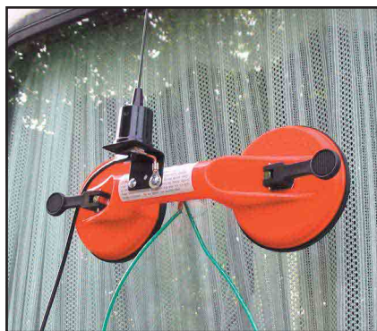
Figure 1—Using a suction cup assembly designed to lift floor tiles and hold glass for transport, the authors, along with KG4JBJ, devised this simple L bracket mount for an NMO antenna.
