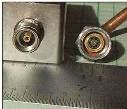
Figure 7—The 3.5 mm connector, female on left and male on right. A black plastic with air holes is used to support the male pin, while the female fingers are suspended in air.
