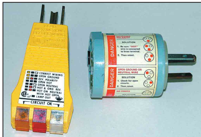
Figure 2 —A pair of utility ac testers. These come in various package styles. The three lights indicate crossed or missing connections and can check more than six possible failure modes. They should be part of every amateur's field/emergency kit.
