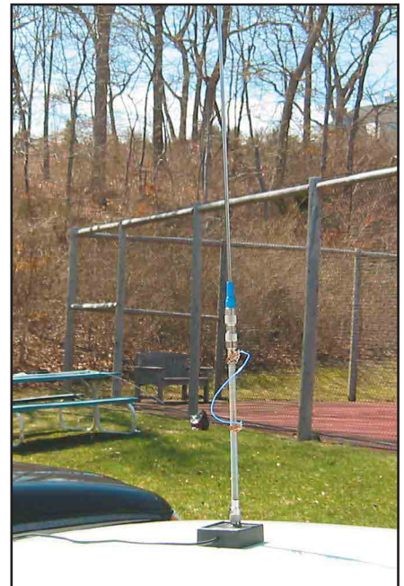
Figure 7—The FARApole used as a stationary mobile antenna with a magnet mount.
