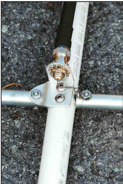
Figure 9—A photograph of the Yagi feed-point assembly. A study of this view and the drawing of Figure 8 should enable easy duplication of the feed system.
