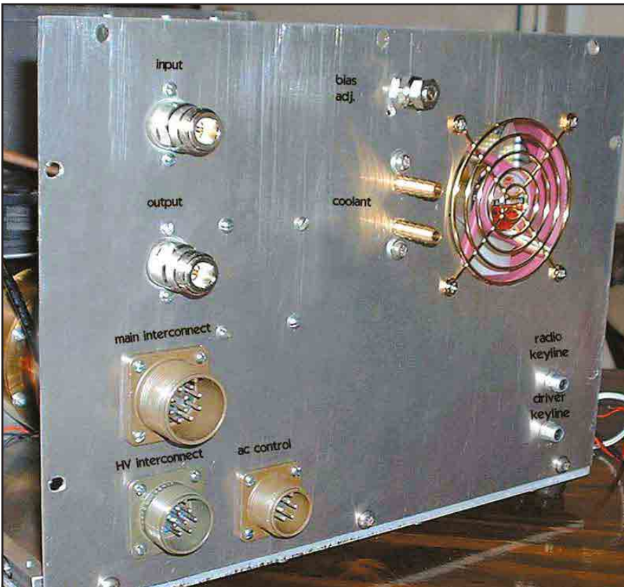
Figure 9—The uncluttered rear panel provides easy access to all connections. Note the use of male power connectors for safety and different styles to prevent connection errors.
