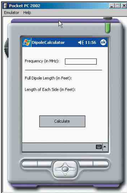
Figure 2—The completed program interface as it appears in the device emulator.
