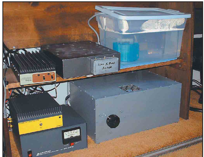
Figure 2 —A small reservoir of water and submersible pump are all that is required to provide cooling for the GS-15B. The amplifier power supply is directly below the container. Be sure to keep the water system safely away from any power sources.
