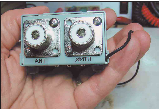
Figure 5—The Tenna Tune back panel.
