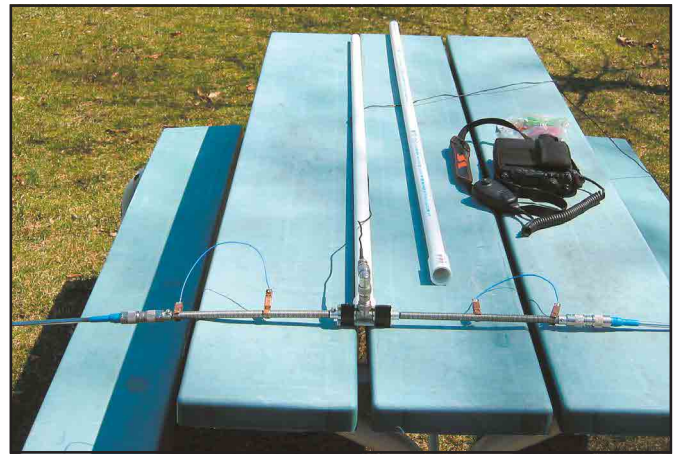
Figure 4 —A dipole version of the antenna can be constructed (see text). The portable mast is made of PVC pipe, joined by a PVC coupling. The elements are mated using a UHF T connector, supported by a PVC T section that is cut in half and joined with electrical tape. One of the elements requires two “B” terminations, as outlined in the text and shown in Figure 1.
