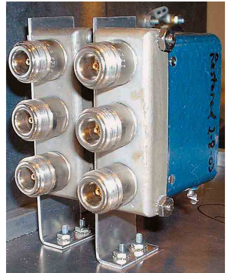
Figure 6—Commercial relays were rebuilt and used for antenna switching.
