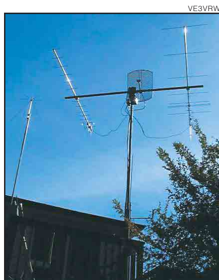
VE3VRW's satellite tracking antennas. Don ports the downlink receive audio to a group of networked repeaters in Toronto. You can listen to the action by connecting to the repeater network via Echolink.
