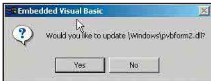
Figure 8—Sometimes eVB will prompt the user to update their DLL files on the target device before the test program will run.
