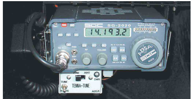
Figure 6—The Tenna Tune installed with the author's SGC-2020.
