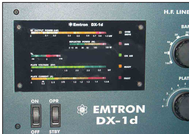
Figure 3—Metering panel of the Emtron DX-1d while on the air from W1ZR.
