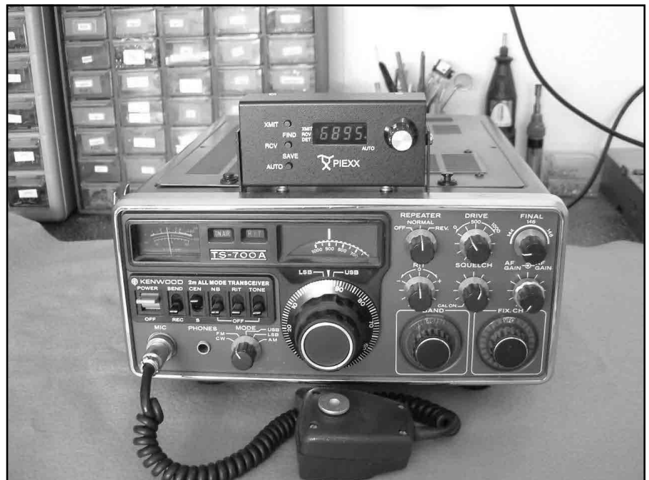
Fig 2—An Uncoder installed on top of a Kenwood TS-700A 2-meter transceiver.
