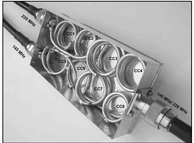
Fig 3—A photo of the 145 MHz/220 MHz diplexer interior.
