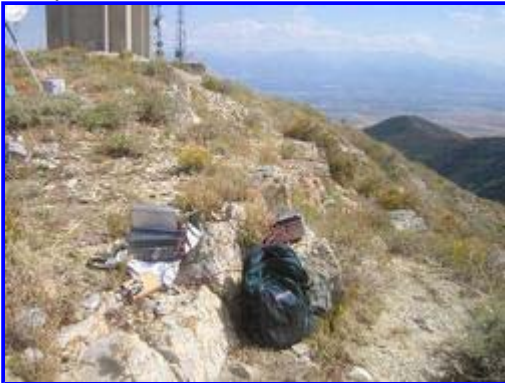
WJ7L's setup. The broader beamwidth helped find Robin's carrier so both ends could improve aim...
