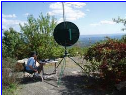
N2UO operating from High Point, NJ. Vegetation is a real problem from this location, unless you can have the dish 20 feet high.
