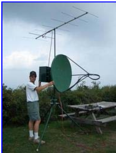
N2UO operating from Camelback Mountain, PA. 20 W into a 40 inch dish. The antenna was very sharp, but all contacts were easy after I set my azimuth with the Packrat's W3CCX beacon.
