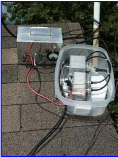
DEMI 2304 Transverter and AMP 20 Watts out, the (melting) lid was left off due to the scolding HOT amplifier.
