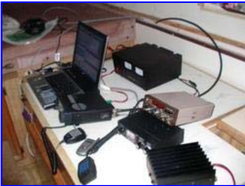
This was the FM Setup, the antenna was on a 100' Fire Tower. It was a Tri-Band Vertical Antenna.
