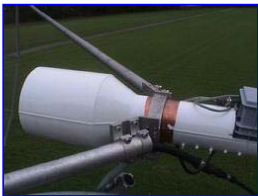
HB9BBD feed mounted at the focal point of his 33' dish
