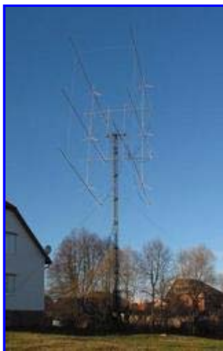
RA3AQ crossed yagi array for 144 MHz EME
