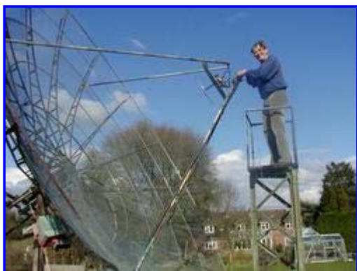
Peter, G3LTF, changing feeds on his 6m polar-mounted dish. He can change bands in about 15 minutes
