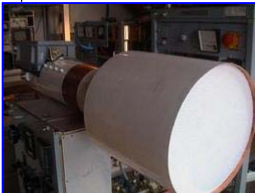
HB9BBD dual-mode 1296 MHz feed ready to go after careful testing in his lab (note the heavy-duty amplifiers in the background)
